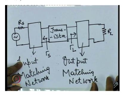
Now when it comes to designing matching networks for amplifiers, let us suppose our amplifier is like this, state has a transistor, some transistor inside it, now your generator will have certain input impedance RS and there will be some load RL.
