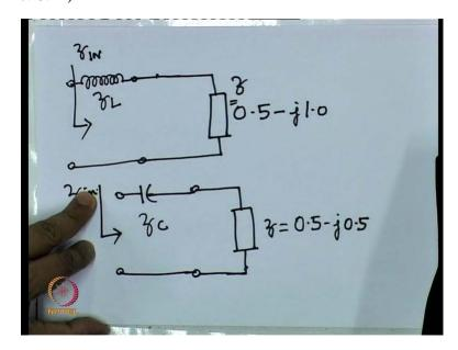
So, when we have an inductor in series, then we move in a clockwise direction upwards. And when we have a capacitance in series, we move in anticlockwise downwards, direction downwards. Let us now consider the case when we have an inductor in, in shunt with the load.
