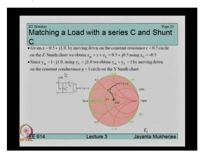
So, at 1<sup>st</sup> we travel along a constant resistance circle and this point is upwards than the origin, so we have to go downward. So, 1<sup>st</sup> what we will do is that will go downwards along a constant resistance circle and then touch the G equals to 1 circle at this point once we touch G equals to 1 circle at this point, we note that if we go along this G equals to 1 circle, we can reach the origin.
