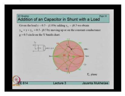
For this again we go to our slides on the monitor and we see that on connecting a capacitance in shunt Y traverses in the anticlockwise direction along constant conductance circle till it reaches the point YN.
