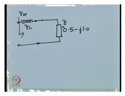
Now suppose we have a load connected let us consider a simple load Z and say it is normalised impedance is this, so this small z is equal to this. And we now connect an inductor in series like this. So, this is an inductor having a normalised impedance zl. So, when we connect this zl, how does the input impedance change.
