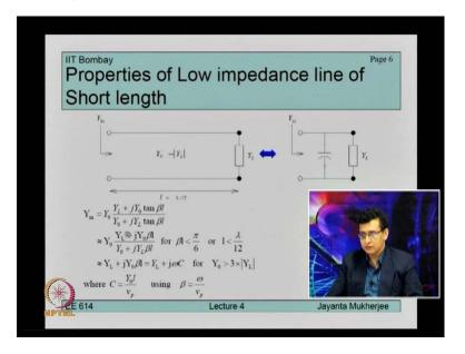
Or if we use lower impedance line i.e. the one that has low value of Z0, then also they can show that it will act as a capacitance because for low value of beta L that is when beta L is
