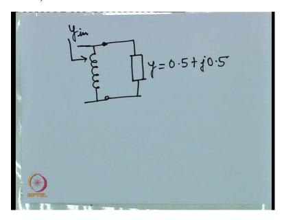
If we have an inductor in shunt, suppose we again have a load Y equal to 0.5+ J0.5 and we connect an inductor in shunt as shown. Then what happens. So, let us go back to our slides on the monitor.
