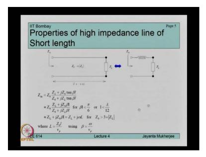
Now if we go once again back to the slides on the monitor, then one common way of implementing a microstrip line would be... Or if we choose a high impedance line of short length, then it can act as an inductor.
