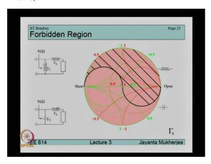
Now it is not always possible to obtain a solution. For example, if we have, if we have a load when we would like to connect a matching network like this that is an inductor in series and an inductor in shunt after that, then is that load is in this region shown by this shading mark, then we see that no value of this load can be obtained on matching network.
