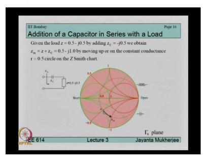
If we go to the slides on screen, we see that this is the initial Z that we had, just like in the previous slide but then on connecting a capacitance in series what happens is that this Z travels and becomes a new value Zin and the locus that we travel when we move from Z to Zin is along a constant resistance circle and in a downward direction.
