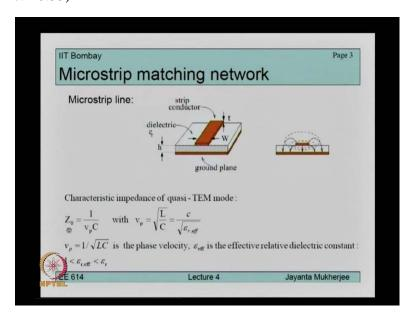
Now microstrip matching network is an example of of a transmission line where the Z0 and BP are given like this. Microstrips are often used for implementing these matching networks.
