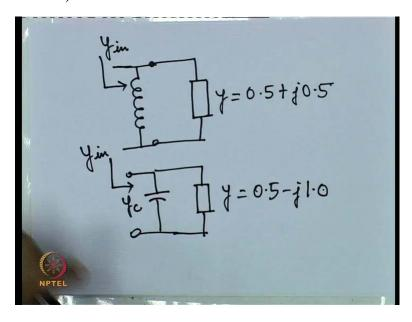
And finally let us consider the case when we have a capacitor in shunt with the load. So, say our Y is equal to 0.5 - J1.0 and this is YC what will YN be.
