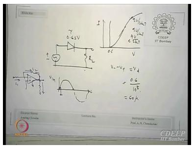
Normally if you have a diode okay load here and a signal here what is the way; say this is a half way rectifier we say so whenever this becomes positive signal the diode conducts okay, diode conducts. So, all of it is transferred to RL okay, whenever this becomes negative now it is reverse biased and no output is seen is that correct. So, we say rectified AC became DC one direction unidirectional.
