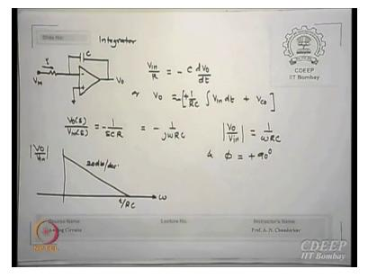
So, without going into much detail for integrator if you see an integrator I have an input register so what do I do an integrator exchange capacitor with a resistor wherever there was a register put a capacitor where ever capacitor put the resistor and it will become inverse V in by R is - c dv0 by dt so V there okay; only thing you should remember in the case of integrator this initial value has to be specified because capacitor may completely charged.
