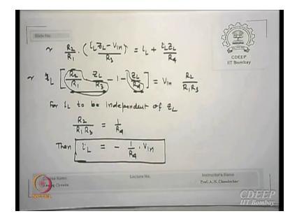
I am going to get iL into R2 by R1 upon 0+ R3 -1-, I just collected iL terms = Vin upon R2 by R1S, now what is the condition I should have that iL should not be a function of ZL, the upper equation shows there is ZL terms appearing is that correct, ZL terms appearing. If I want iL to be only functions of resistances okay independent of ZL what is the condition I should meet that R2 by R1 R3, R2 upon R1 R3.
