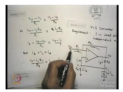
I am now trying to get the current equation V in - VL. Please remember V- is VL, so V in - VL by R1 is VL - V0 by R2 which is the current flowing from this that card I1 and I2 are equal. So, I1 is V in - VL by R1 and I2 is VL - V0 by R2 they are equal.
