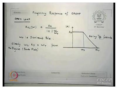
So, we were looking for frequency response which is essentially for any amplifier or any system is interesting. if you have an OPAMP which is an open loop case then the open loop gain is A0 upon1+ j by Omega 0 this is a transfer function for a normal open loop amplifier okay, OPAMP (FL) gain is falling 20 log V2 by V1 after Omega 0 and at 0 the gain is DC gain which is A0, this is the transfer function of open loop OPAMP and therefore Omega 0 is the dominant pole. (FL)
