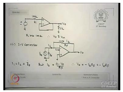
One of the use of a OPAMP is to convert of what I should say V to I converter or I to V converter and see the typical current to voltage converter you have a current source and obviously we know in the OPAMP, if it is in the negative feedback system and the V+ is grounded the current entering here from the current source must enter through RF because no current can enter OPAMP why we say so.
