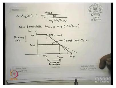
Now if I substitute this back into my closed loop this then this = 1 ACL 0 upon1 + J Omega upon this okay. So, what is the new bandwidth now, we substitute (FL) Omega naught into A0 by ACL 0 (FL) is that correct, let us see what we are done. If you have a open loop this was your amplifier Bode plot is that correct. If I have a closed loop the ACL 0 is the DC gain okay and it has a pole of Omega CL0 which is here Omega 0 times A0 by AC and 0 (FL)
