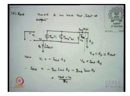
The second term in the gain function was r out and please remember our route is essentially the net output resistance, but right now we first calculate the output resistance other than the load because as seen from the drain side. So, we calculate R o from here, what is the condition there to calculate output resistance put a voltage source at the output and short all independent sources the standard technique of Kirchhoff circuit analysis short all in independent sources.
