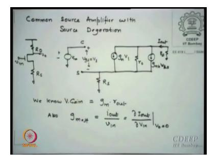
This is an interesting amplifier which shows that there is a resistance in the source and it is very popularly known as source degeneration. Now why this is relevant at times may be shown when the output appears for this amplifier, this is the kind of equivalent circuit which I draw from the razavis book this is not mine.
