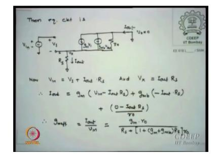
So, first thing we do is we want to find gm effective. So, we will make V 0 0 and put V in and find I out by V in that is the standard technique to find gm. So, I put V 0 equal to 0 is that correct I is equal to g m Vn plus go ro go V out itn is equal to I by V in is that what we said it. So, I make V 0 0. So, I ground this output is that clear as soon as I ground output there is no current in the RD. So, I just forget about RD. So, I have gm 1 V 1 gm V 2 Vbs plus r 0.
