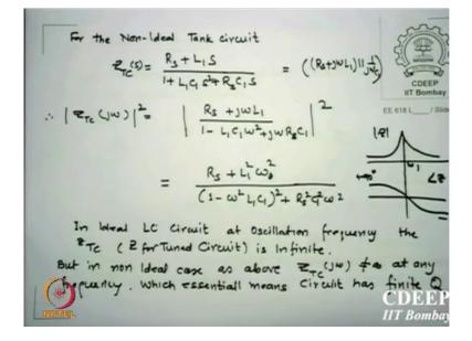
So, I calculate it RS plus L1 S upon 1 plus L1 C1 S square plus RS C1 j omega 1 and RS are in series and parallel is a capacitor. So, if I do this this is what essentially RS plus j omega l, parallel to 1 upon j omega see if you expand this I get this terms and if I evaluate the value of this at square. So, I can say magnitude of this can be RS L1 square omega square 1 minus omega square L1 C1 square this is a complex quantity magnitude were real magnitude wise this value will appear.
