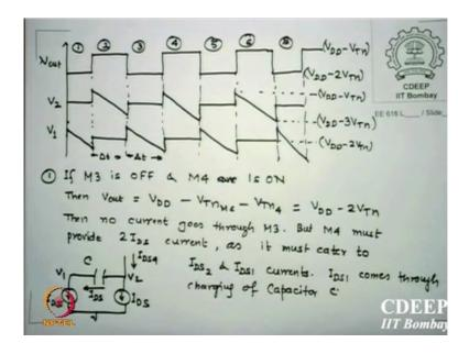
So, that happens I have a figure you can draw that; I do not I can keep this you have the figure I do not have, but I can keep like this. So, I am interested to know these 3 potentials here, here and here. V1 V2 and v out, v out bar is the bar of that. So, that we can just see the otherwise; think of it, if this potential should be at least and they are equal if this device has to be switched off it should be at least one V T below.
