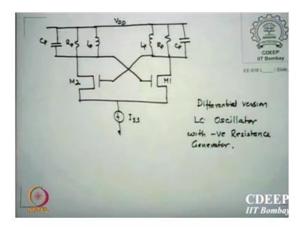
But you can see from here these and these 2 transistors are. So, connected the actually are providing negative impedance at these 2 terminals 1 by 1 think of it.
