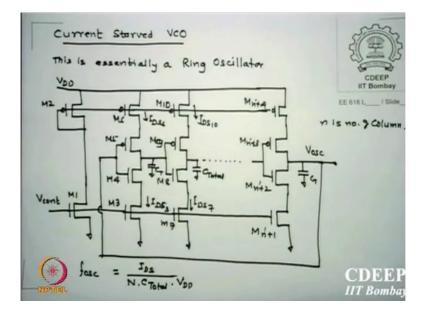
Now, it is also called current starved VCO. This M1 M2 essentially forms a mirror kind of input side. So, and that is controlled by V control. So, if I have on M1 if I decide my V control I decide the current in M1, and since it is made on that wherever I connect the same
