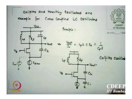
I have one transistor here I have one CP across the tank circuit and I have another capacitance between output to this and please remember here, what is this transistor is working like?
