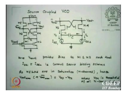
Which is the most common VCO, also popularly known as multivibrator; because we have got mostly on the bipolar circuits you will not immediately guess this is same circuit, but it is essentially a multivibrator. And implemented in cmos technology or nmos technology. If it is a this is all nmos, if I wanted to make a cmos transistor m 5 and m 6 p channel gate ground.
