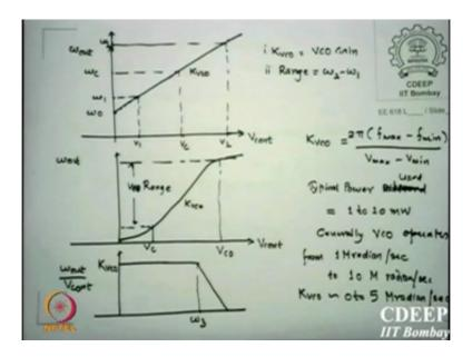
Now, what are the features of a VCO if I plot the same curve which I just now same expression w out versus v controlled. I have linear relationship that means, k is treated constant. I may vary the k, but k is slope which is constant; that means, I can do this, but forgiven this k VCO is there giving a slope for this curve, y is equal to mx plus c. This is the frequency omega 0.
