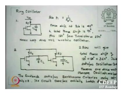
Yeah, that we can read in a second-year book this is just main important part you should look if you have a signal transistor and you have a single capacitor, which may be the cdb of the transistor itself and may be some output into wire connections. Then we see it has a single pole it has a single pole which is 1 upon Rd Cl.
