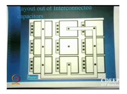
Instead of having a large capacitors you can actually create small capacitors of C 1, C 2 or C 1 and then connect in a fashion well do you see this capacitance is not connected to anywhere these are connected 6, 6, 2, so 8 capacitances if are connected to give 8. Let us say this has the capacitance of 1 or C this is 8 C is that clear. This is c and this all are in parallel made, so they are 8 C.
