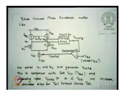
A typical CMFB this circuit is shown here this is your diff amp and this I DS 3, I DS 4 are coming from some BBN mirror as we did. I actually do one thing I figured out what is V o 1 and V o 2. So, I must first sense them. So, there is some circuit which is called common mode sense circuit. It figures out what is the V o 1 and V o 2 values, them some those to values it generates what we called as would CMFB voltage V CM. Then we
