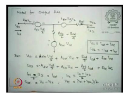
By similar argument I can put an equivalent T network or the output of a different fully differential system. And again I can get V o 1, V o 2, V o d and V o c accordingly, this is what has been done. And using this we will be able to calculate A cm and A dm for a fully differential amplifiers. Please remember I am sorry I am not able to spend time on this because they are lot many things to be done, but I am going to posted, so you can look all of it.
