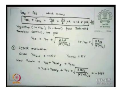
So, an individual arm of a diff amp the IDS 1 and IDS 2 will be the half of this current, which is 12.5 micro amps
