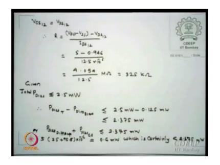
So, [FL] expression [FL] r is equal to VDD minus Vss minus VDS 12 into this, which gives me a value of 3 25 kilo ohms to get the currents are 12.5 micro amps. I need for this W by L are 4, I need a size of register of 3 25 kilo ohms bias [FL] power [FL] 0.125 available [FL] 2.5, the diff amp plus [FL] available a 2.375 milliwatts is still available for me for the limit for diff amp plus gain stage bias [FL]
