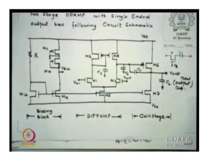
The Vm essentially is, if I calculate from here it is Vss plus VDS sat 5, this voltage plus this voltage plus VGS of 1 is that clear
