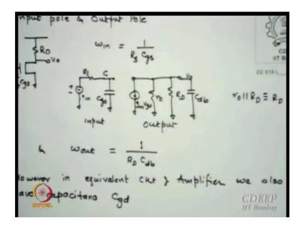
What will happen rd parallel or 1 gm or r 0 r parallel whatever it comes corresponding loads will appear, as of now rd represents load whichever way you create, first in this say if this is your this and we right now mid light there is a capacitance between gate and drain in a normal transistor which is called C g d, which is very important capacitance, right now I am not shown it.
