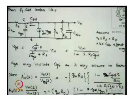
So, here is the equivalent circuit of a mass transistor amplifier common source, I am applying a input signal through a series resistance of the source R s.
