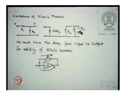
So, there is a gain equivalently gain, but; however, if I make a transformation by the 2 Z 1 Z 2 functions, on the one side I get R 1 plus R 2 which is as good as many input this is there in a.
