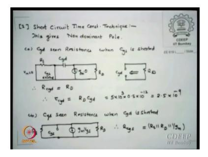
This is the dominant lower frequency. So, revis[ion]- is note down f p 1 is 3.68 mega hertz if tau 1 tau 2 calculate oh substitute the next step for the capacitance you are really looking for, let us say I want to find resistance seen by C g d. So, capacitance physically short. So, as soon as I short this a shorted rs short means short.
