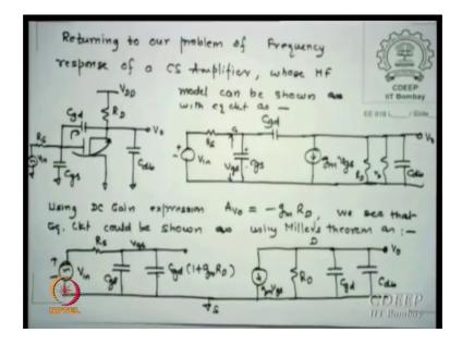
So, return into our problem of frequency response common source amplifier, a typical common source amplifier is here, equivalent circuit is shown here, the dc gain is here marked d and using the milers theorem now I can replace.
