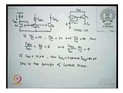
Here is some interesting features how mirrors are used, the mirrors are used to create currents in different arms. So, it need not be of the same current in different places. So, I may actually have this R M 1 based calculation to give me I DS 1, and then I can have W by 1 differently for M 2, M 3 as long as I connect their gates V GS 1 is equal to V GS 2 equal to V GS 3. And in that case, the ratio of this to this is W by L, ratio of this to this
