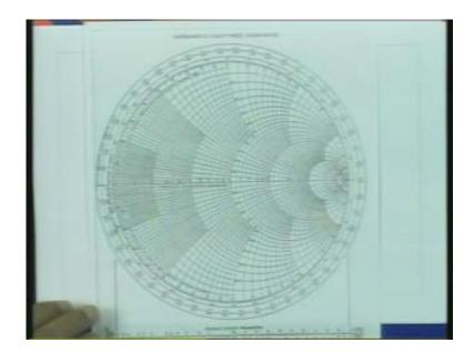
So as we can see here this circle is the unity circle, this is the real axis of the gamma which is u axis, the center here is the origin of the complex  $\Gamma$ -plane. These circles which are flaring like that, they are the constant reactance circle and this circle which are one within another represent the constant resistance.
