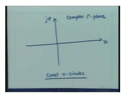
So as we saw the center for this circle is  $\frac{r}{r+1}$  so the center is  $(\frac{r}{r+1},0)$  and the radius for this circle is equal to  $\frac{1}{r+1}$ .
