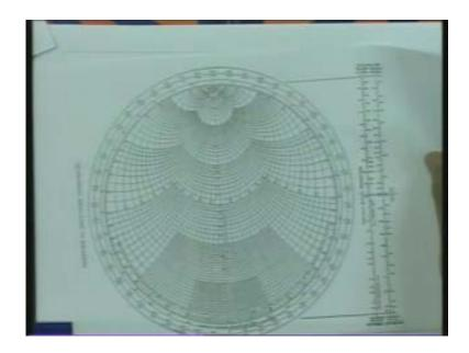
We should keep the smith chart like this so that the complex reflection coefficient axis is properly defined.
