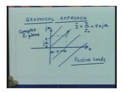
As we have seen earlier, the reflection coefficient  $\Gamma=\frac{Z-Z_0}{Z+Z_0}$  where  $Z_0$  is the real quantity for a lossless line, Z in general could be complex if I write this expression in the normalized impedances I can take  $Z_0$  common from numerator and denominator so this
