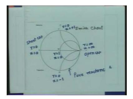
So when the impedance lies on the center of the smith chart which corresponds to the magnitude of the reflection coefficient zero then this point represent the matched condition on the Transmission Line.
