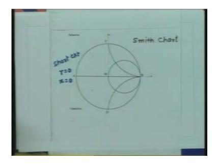
Similarly if I go to the other point here b as we saw the two sets of circle degenerate into a point and that is this point so this point corresponds to  $r = \infty$ , it also corresponds to  $x = \infty$  so this point here is  $r = \infty$ , it is also  $x = \infty$ . That means the impedance is infinity so this point is nothing but the open circuit point, you have this circuit which is the open circuit point.
