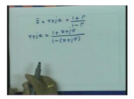
So I will get r equal to some function of u and v, similarly x equal to some function of u and v. So from this relation I will get two equations on the complex gamma plane for a given value of r or x. Essentially when I map the impedances on the complex gamma plane I will see two set of curves on the complex gamma plane one will correspond to a given value of r other will correspond to a given value of x.
