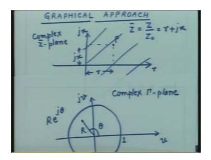
So for doing this transformation let me go back again to the original relation which I had and that is the impedance I can write as normalized impedance  $\overline{Z} = r + jx$  that is equal to  $\frac{1+\Gamma}{1-\Gamma}$ , substituting for  $\Gamma = u + jv$  I get r + jx that is equal to  $\frac{1+(u+jv)}{1-(u+jv)}$ , I can rationalize this function and separate out the real and imaginary parts.
