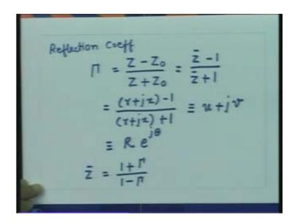
So this transformation between the reflection coefficient and the normalized impedance is a one to one transformation.
