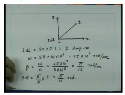
And we can just get this quantity beta t omega t that is equal to 2pi into 10 to the power 7 into 1 microsecond which is 10 to the power minus 6 so that is equal to 20pi radians.
