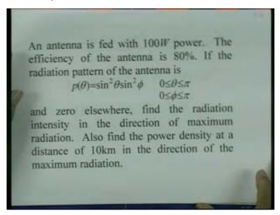
There is an antenna which is fed with 100 watt of power. The efficiency of the antenna 80 percent. if the radiation pattern of the antenna is given as p theta equal to sin square theta sin square phi where theta varies from 0 to pi and phi varies from 0 to pi and 0 elsewhere find the radiation intensity in the direction of maximum radiation. Also find the power density at a distance of 10 kilometer in the direction of maximum radiation.
