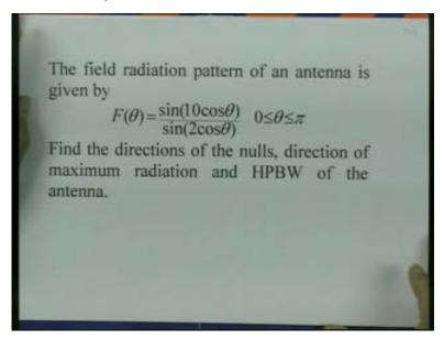
Let us now take a problem which is a general problem for the antenna and that is the field variation pattern of an antenna is given by F theta which is equal to sin of tan cos theta divided by the sin of two cos theta where theta varies from 0 to pi. Find the directions of the null, direction of the maximum radiation and also the half power beam width of the antenna.
