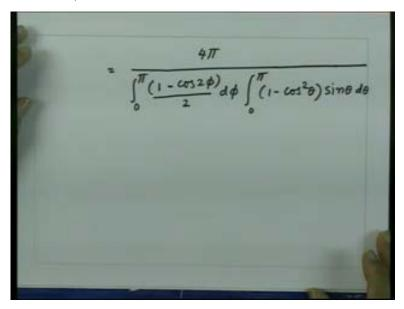
Now in this integral we can substitute for cos theta equal to t so sin theta d theta will become dt, this integral is now very simple to solve so you get finally a value which is 4pi divided by pi upon 2 that is 2 upon 3 this value. So you get a directivity for this antenna which is 12.
