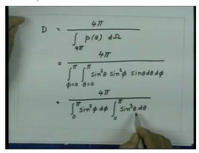
This integral we can solve by expanding this in cosine of 2 phi and this one we can write as 1 minus cos square theta and sin theta so these two integrations can be written as... this is 4pi from 0 to pi this you can write as 1 minus cos of 2 phi upon 2 d phi so the sin
