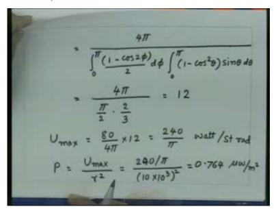
Once we know the the power density then we can find out the electric field at the point because the power density P is mod of E square divided by eta so E electric field will be equal to square root of power density into eta is equal to square root of 0.764 microwatts per meter square so this is 10 to the power minus 6 for microwatt into eta which is 120pi. So simplifying this essentially we can get the expression or the value of the electric field at that distance.
