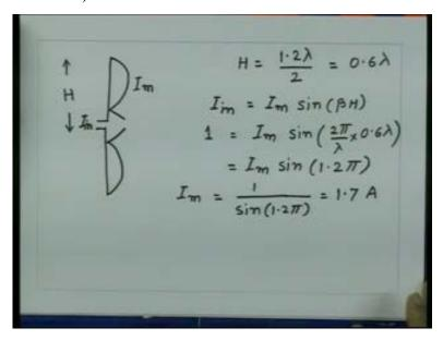
Once we get this quantity I m then we know that this dipole for the radiation field that is only theta component E theta and that is equal to 60 I m upon r where r is the distance measured from the center of the dipole, cosine of beta h cos theta minus cos of beta h upon sin of theta.
