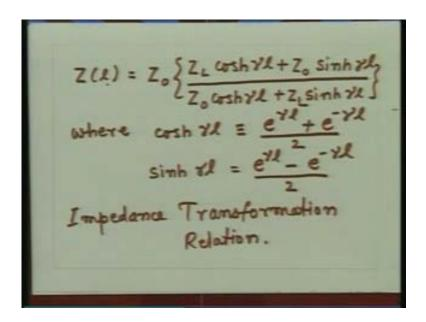
And we have seen the impedance is given by this Z at any location 1 is equal to the characteristic impedance multiplied by this impedance transformation term, where this quantity is the hyperbolic cosine and hyperbolic sine which are given in terms of the propagation constant  $\gamma$  and the length on the Transmission Line.
