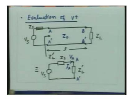
I can put the lumped circuit analysis and find out what is  $V_A$ . So,  $V_A$  will be  $\frac{Z'_L}{Z'_L + Z_S} \cdot V_S$  and  $I_A$  will be  $\frac{V_A}{Z'_L}$ .
