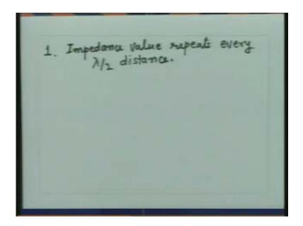
Going back to this expression here let us say I have a impedance value of Z(1) at some location on the line now if I move by a distance of  $\frac{\lambda}{2}$  from here that means if I go to a location  $1 + \frac{\lambda}{2}$  then the impedance at that location would be where I will be replaced by  $1 + \frac{\lambda}{2}$
