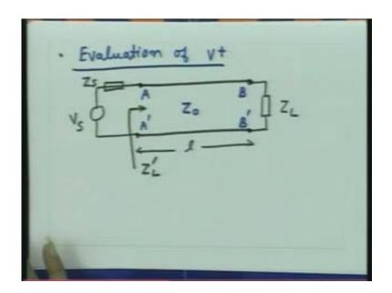
Once I transform the impedance then the whole circuit is the lumped circuit at this location I do not have to worry about the distributed elements. so now this circuit is equivalent to having a voltage source which is  $V_S$ , the internal impedance for the voltage source that is  $Z_S$  and connected to a effective impedance which is  $Z_L$ , once I get that then I can find out what is the voltage this is the location now A, A' so by using the lumped
