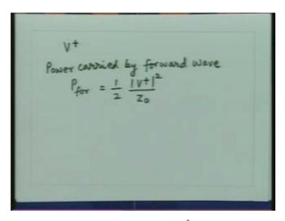
So the power delivered to the forward wave is  $\frac{|V^+|^2}{Z_0}$  where  $\frac{1}{2}$  is the factor for the rms value of the power.
