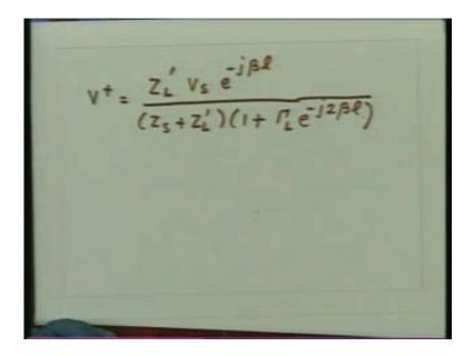
Once I know the value of  $V^+$  then my problem is completely solved I can substitute that in to the power calculation and I can find out what is the power delivered to the load or what is the power at any particular location on the line.
