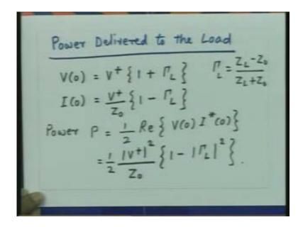
So the power delivered if I knew the value of  $V^+$  then I can find out what is the power delivered to the load, how do we find out  $V^+$  which we will discuss in a minute. However at this location if I know the amplitude of the forward traveling wave and if I know the load impedance I can calculate the value of the power delivered to the load.
