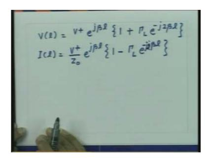
Now again as I did in the previous case at the load point I have the voltage and current so the total power the complex power P at that location I is equal to ½ (V I\*) I can substitute from here for (V I\*) and I get ½  $\frac{\left|V^{+}\right|^{2}}{Z_{0}}$  {1 +  $|\Gamma_{L}|^{2}$  + 2I<sub>m</sub> ( $\Gamma_{L}$  e<sup>-j2 $\beta$ I</sup>)}. It is simple algebra you substitute the value of V and I in the expression here you get the complex power which will be essentially given by this.
