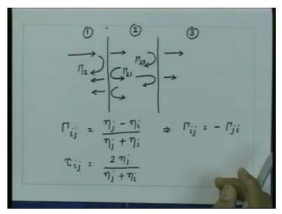
So now if I if I write down and you are having this distance d and the phase constant in this medium let us say is given by beta so you are having the phase change when the wave travels from here to here which is equal to corresponding to beta d. So this wave
