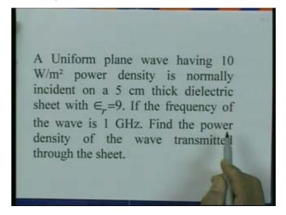
Here we have a uniform plane wave having 10 watts per meter power density is normally incident on a 5 centimeter thick dielectric sheet with epsilon r equal to 9. If the frequency of the wave is 1 gigahertz, find the power density of the wave transmitted through the sheet.
