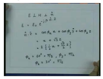
So one one thing we can note from here that since the phase function has only x and z terms in this essentially the wave is propagating in the xz plane and that is what essentially we see here that the wave normal makes an angle 60 degrees with the x axis, 30 degrees with the z axis and 90 degrees with the y axis that means the vector lies in the xz plane.
