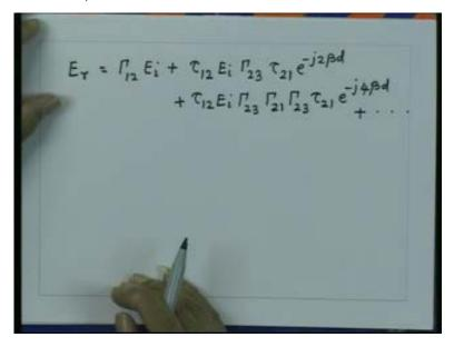
So essentially you see if I take this quantity common you will have now a geometric series for this. so we can write down now the reflected wave E r that is gamma 12 E i plus tau 12 gamma 23 tau 21 e to the power minus j beta d into 2 and summation of the geometric series which we get for this term will be multiplied by E i upon 1 minus gamma 12 gamma 23 e to the power minus j 2 beta d.
