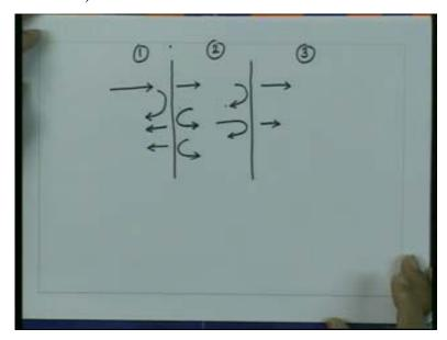
Now if I say that the reflection at i j boundary so that means 1 2 boundary if I take that would be gamma 1 2, so from here let us say reflection I write down at an interface which is given by i j that is nothing but impedance of the medium j minus impedance of the medium i divided by impedance of the medium j plus impedance of the medium i and from here essentially we get gamma ij is equal to minus of gamma ji.
