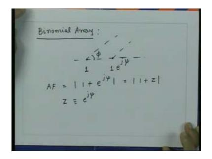
Now for this array we have a null when z is equal to -1 so when this quantity goes to zero we have nulls. So for this array the null correspond to z is equal to -1 that is e to the power j  $\psi$  is equal to -1. So whenever this condition is satisfied you get the null in the radiation pattern.
