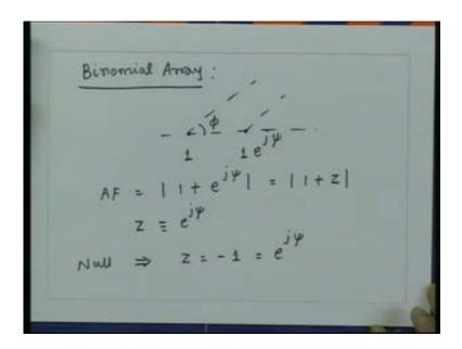
So if I consider an array factor which is one plus z to the power N we get the new array factor which is one plus z to the power N so if I expand this now binomially I will get this is one plus  $Nc_1$  z plus  $Nc_2$  z square plus and so on with plus  $Nc_N$  z to the power N. As we discussed in the last lecture if I take the coefficients of z they essentially give me the
