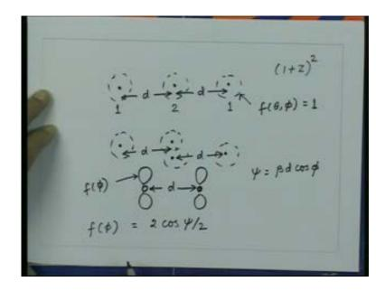
So the total pattern which we get for this binomial array will be equal to  $f(\emptyset)$  multiplied by the array factor which is equal to two times  $\cos\psi/2$  multiplied by again the array factor which is  $\cos\psi/2$  so we get a radiation pattern which is two times cosine square of  $\psi/2$ .
