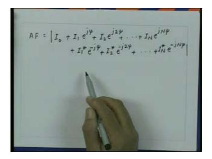
Now we can combine the terms of this and noting that this  $I_1$  e to the power j  $\psi$  and  $I_1$  conjugate e to the power -j  $\psi$  are complex conjugate of each other we can write this array factor as  $I_0$  plus  $I_1$  e to the power j  $\psi$  plus  $I_1$  e to the power j  $\psi$  conjugate this gives me  $I_1$  conjugate e to the power -j  $\psi$  plus so on and the last term would correspond to  $I_N$  e to the power j  $\psi$  plus  $I_N$  e to the power j  $N\psi$  conjugate.
