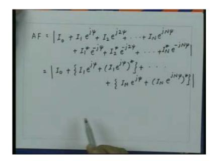
Now this thing can be combined together this is the quantity which is  $I_1$  e to the power j  $\psi$  and the conjugate of conjugate of that. So this essentially gives the real part of this quantity two times the real part of this so we can write down the array factor as  $I_1$  plus two times real part of  $I_1$  e to the power j  $\psi$  plus two times real part of  $I_2$  e to the power j  $\psi$  plus and so on two times real part of  $I_N$  e to the power j  $N\psi$ .
