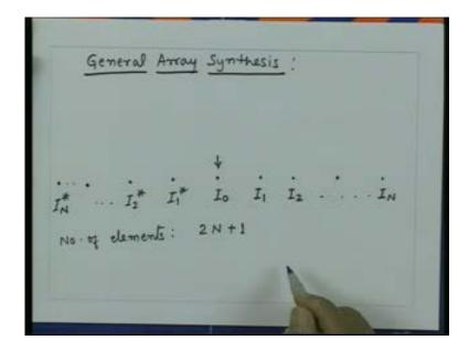
We are assuming essentially there is an array which is having odd number of elements and there is symmetry in the current distribution in the sense that the amplitude of the currents is symmetric and the phases of the currents are antisymmetric. So if this phase is delta this will be minus delta and so on. Now this quantity is here I so I can write down in terms of real and imaginary parts. So explicitly we can say that current of let us say K th element is  $I_K$  is given by  $a_K + jb_K$ .
