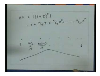
We can look at this in a little different way from our basic the analysis of the array. Now let us consider a three element array which is having binomial coefficients so let us say we have three elements which are having three elements binomial array so this would correspond to essentially one plus z square that is what the polynomial would be so the coefficient for this would correspond to one two and one these are the binomial coefficient for one plus z square.
