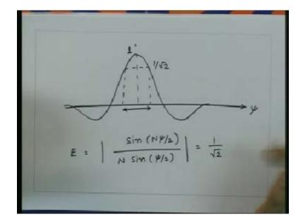
So for a approximate calculation of the half power beam width what we can do is we can find out the directions of the nulls from there we can find out the beam width between the first nulls and then we say the half power beam width is approximately half of the beam width between the first nulls. So we essentially say that approximately the half power beam width is equal to the beam width between first nulls divided by two.
