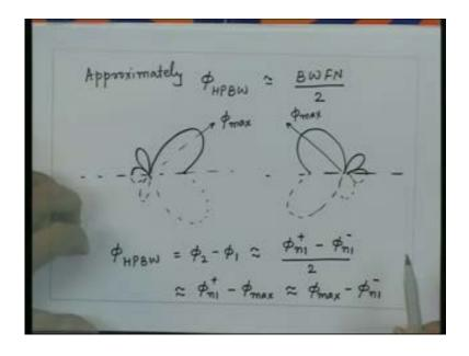
So if I consider any nulls in this case this would correspond to  $\emptyset_{n1}$  to the power minus this would correspond to  $\emptyset_{n1}$ to the power plus so this angle is approximately equal to the half power beam width the same is true here this angle corresponds to the half power beam width.
