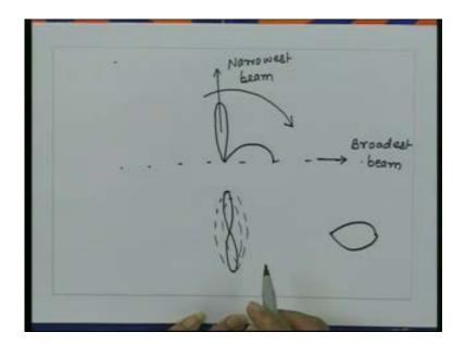
So in one case though the beam in the planar looks only change in shape for change in the half power beam width if I visualize the radiation pattern in three dimension the radiation patterns are quite different in two situations the end fire will look more like a balloon like that where the broad side would look more like a flat disc which is figure of revolution in this direction.
