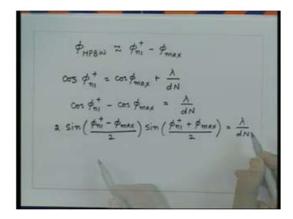
Now if N is very large the half power beam width is much much smaller than one because the beam width between the first nulls is going to be very small. So if I say that if
