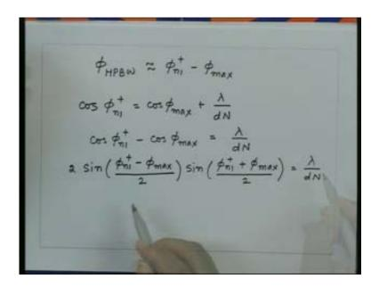
Now this quantity as we said is nothing but half power beam width so I can substitute now for  $\phi_{n1}$  to the power plus as the half power beam width plus  $\phi_{max}$  so this one can be written as two times  $\sin(\phi_{HPBW}/2)$  into if I substitute for this which is  $\phi_{max}$  plus phi half power beam width it will be  $\sin[(2 \phi_{max} + \phi_{HPBW})/2]$  that is equal to  $\lambda/dN$ .
