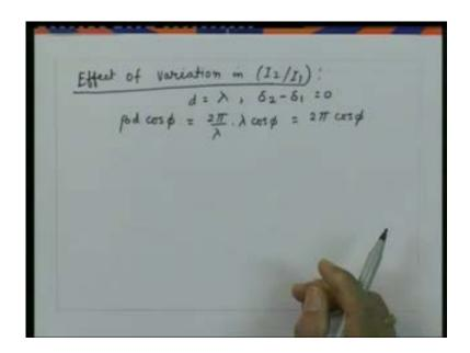
I can substitute into the general expression for the radiation pattern so we get E that is  $K_0$  and again you can assume delta one is equal to zero and  $I_1$  is equal to one without loosing generality. So this quantity then  $I_1$  e to the power j delta one will be one so this is  $K_0$  into one plus this ratio  $I_2/I_1$  where  $I_1$  is one so e to the power j  $\beta$  d cosø will be  $2\pi \cos \theta$ .
