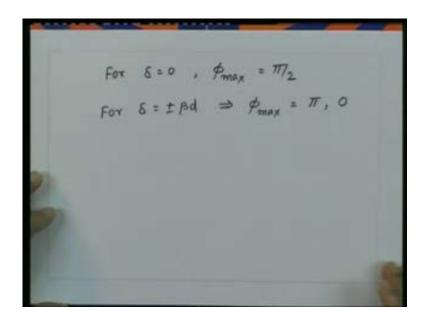
So what we note here is as we change the value of delta the beam maximum direction is changes from zero to  $\pi/2$  to  $\pi$ . So as the angle changes from  $-\beta d$  it corresponds to zero to  $\pi/2$  when delta is zero and when delta becomes equal to  $+\beta d$  the maximum direction is going to  $\pi$ .
