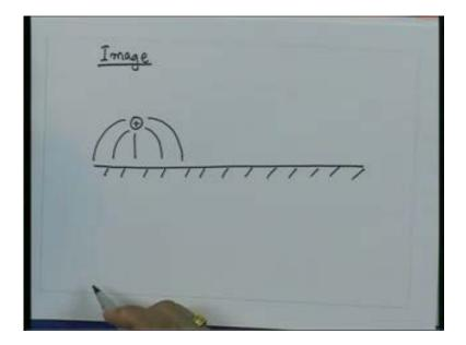
So the ground plane can be replaced by an image charge so this thing is essentially equivalent to putting a negative charge here and then replacing the ground plane, or we can say conversely if you have the positive and the negative charges we can say this is equivalent to having a charge and a ground plane, precisely that is the fact we make use of when we investigate the characteristics of a monopole antenna.
