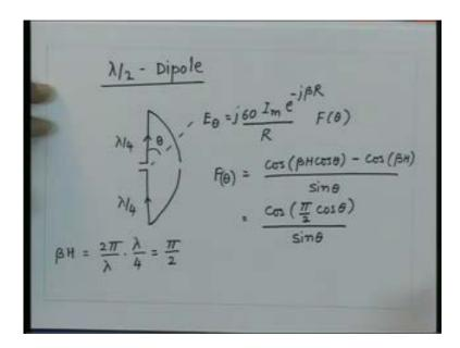
Now as we have seen it has only the nulls which are in the direction along the axis of the antenna it is also maximum in  $\theta = \pi/2$  this quantity is zero so this is one so you get the maximum field which corresponds to  $\theta = \pi/2$  so its radiation pattern we had seen looks like similar to the Hertz Dipole it has only maximum perpendicular to the axis of the dipole and the field is zero in the axis of the dipole.
