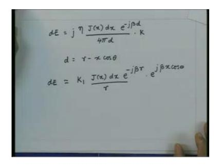
So the total electric field is nothing but integral over the length of this current distribution so I get the total electric field E that is integral zero to I this quantity  $K_1$  e to the power -j  $\beta$  r upon r that is constant for given distance J(x) dx e to the power j $\beta$  x cos $\theta$ .
