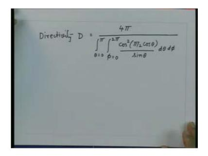
As we know the value of this integral over  $\theta$  is 1.218 so this directivity is equal to  $4\pi$  upon the integral over  $\theta$  which is  $2\pi$  and integral over  $\theta$  is 1.218 so the directivity of the half wave dipole is about 1.64, as we mentioned earlier the directivity is given in terms of dB's so we can take 10 log of this quantity so it will give you the directivity in dB's so we get D in dB's that is 10 log 1.64 and that will be approximately equal to 2.15 dB.
