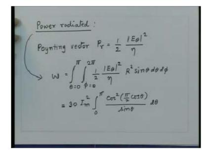
Note here the  $I_m$  is the maximum current which you see on the dipole and in this case since the length of the dipole is  $\lambda/4$  this is the current which is  $I_m$  so this value of current is essentially  $I_m$ . So in general dipole the maximum current need not be at the internal terminals but if you take a dipole which is  $\lambda/2$  long then the input current is the maximum current which you can see in the dipole.
