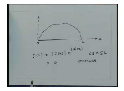
We can think of this current as small small current elements so I discretise this current distribution in the small elements and let us say I have a small current element here which is at a distance x so the current which is flowing into this is the linear current density which is the J(x) times dx if the width of this current element is dx. So the current which is flowing in this direction is J(x) dx so that is the current in this which is J(x) amplitude now J(x) into dx.
