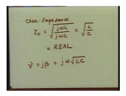
So we have  $\gamma=j\beta$  that is again equal to  $j\omega\sqrt{\frac{C}{L}}$ . Now with these parameters we will again revisit the voltage and current expressions on Transmission Line and then we carry out the analysis of the standing waves on the Transmission Lines.
