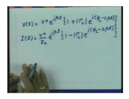
Now let us see how the voltage and current varies if I measure the magnitude of the voltage and current along the Transmission Line, what is the variation of the voltage and current along the Transmission Line.
