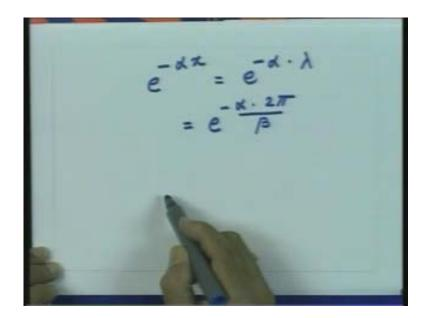
Since for low loss condition  $\alpha$  is much smaller than  $\beta$  this quantity  $\frac{\alpha.2\pi}{\beta}$  is much less
