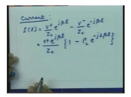
These two terms as we know essentially represent the forward and backward traveling wave so the whole expression here essentially represent super position of the forward and the backward traveling wave which is nothing but a standing wave on a Transmission Line.
