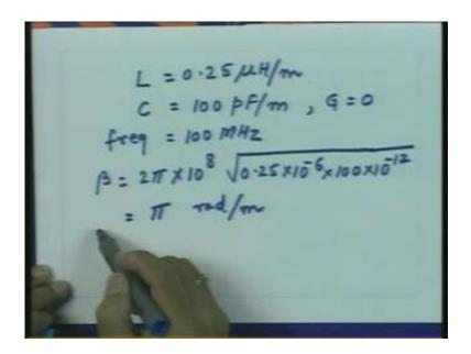
Just to take a number if I say  $\alpha$  is less than one percent of value of  $\beta$  then I can treat the line as the low loss transmission line. The  $\alpha$  should be approximately  $\frac{\pi}{100}$ . Now I can go back and substitute this value of  $\alpha$  in the expression for  $\alpha$  that is  $\alpha = \frac{1}{2}R\sqrt{\frac{C}{L}}$
