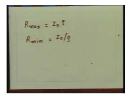
Similarly at the location where the voltage is minimum the impedance measured will be  $R_{min}$  and that will be the characteristic impedance divide by the voltage standing wave ratio. Now if you recall we had mentioned that if the impedance is known on any point on Transmission Line then you can always transform that impedance to any other location on the Transmission Line. Then immediately it strikes to us that knowing the location at
