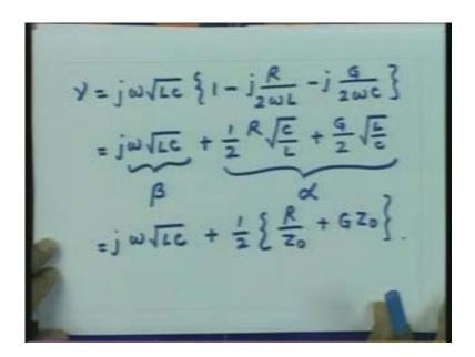
So now the  $\alpha$  can be written in terms of this substitution so I get this value of  $\alpha$  which is equal to  $\frac{1}{2}\frac{R}{L}\sqrt{LC}$ . Similarly multiplying by  $\sqrt{C}$  in the numerator and the denominator in the second term we get  $\frac{1}{2}\frac{G}{C}\sqrt{LC}$ . Multiplying numerator and denominator by  $\omega$  this can be written as  $\frac{1}{2}\frac{R}{\omega L}\omega\sqrt{LC}+\frac{1}{2}\frac{G}{\omega C}\omega\sqrt{LC}$ .
