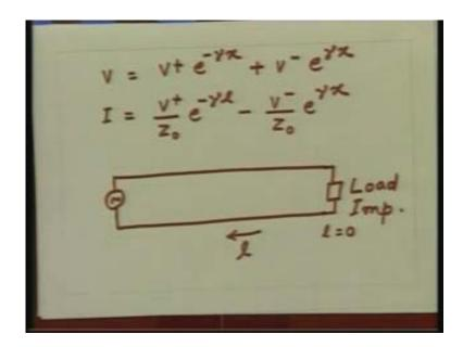
the voltage and current equation can be given by this. This represent the forward traveling wave, this represent the backward traveling wave and now we will replace this quantity  $\gamma$  by  $j\beta$  where x will be replaced by -1.
