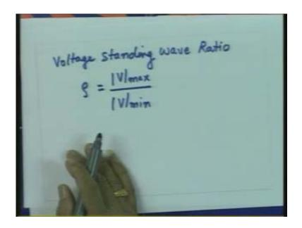
And what is the maximum value of voltage which I can see on the line is  $|V^+|\{1+|\Gamma_L|\}$  and the minimum value which I can see on the Transmission Line is  $|V^+|\{1-|\Gamma_L|\}$ .
