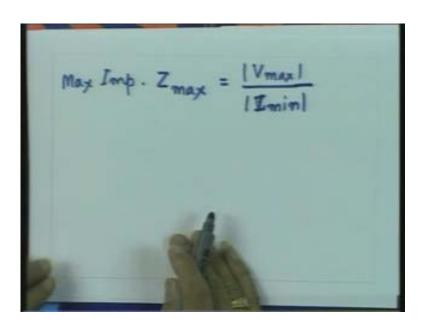
And since we have seen that this quantity when you are having the voltage maximum and current minimum that time the phase difference between them is zero so this quantity is
