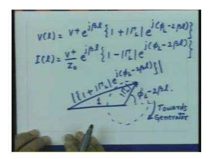
The first term is this vector which is unity the second term is this vector which is rotating as we move towards the generator on the Transmission Line and the magnitude of the total quantity here essentially varies as we move on the Transmission Line. Now the thing to note is when it moves on a circle at some phase when this quantity is zero or  $2\pi$  or  $4\pi e^{j0}$  or  $e^{j2\pi}$  or  $e^{j4\pi}$  that is equal to +1.
