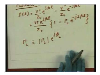
Then I can write down the current and voltage explicitly in terms of this magnitude of reflection coefficient and the phase. So finally I have two expressions here one for voltage  $V(l) = V^+ e^{j\beta l} \{1 + \Gamma_L e^{j(\phi - 2\beta l)}\}$  and the current I(l) will be  $\frac{V^+}{Z_0} e^{j\beta l} \{1 - \Gamma_L e^{j(\phi - 2\beta l)}\}$ . (Refer Slide Time: 20:40 min)
