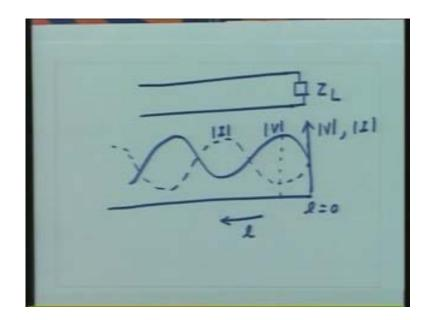
So in this location I get voltage maximum and current minimum, when I go here I get current maximum and voltage minimum. The important thing is when the standing waves are present on the Transmission Line then the voltage and current waveforms are shifted with respect to each other and maximum of voltage aligns with minimum of current and vice versa.
