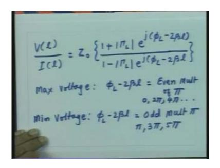
So when the voltage is maximum this quantity is +1 so  $Z_0$  is real, now this quantity is one  $|1 + \Gamma_L|$  denominator this quantity is again +1 so this quantity is  $|1 - \Gamma_L|$  so the ratio of this quantity is the real quantity. When the voltage is maximum the impedance seen on the Transmission Line is real irrespective of what the line is terminated in.
