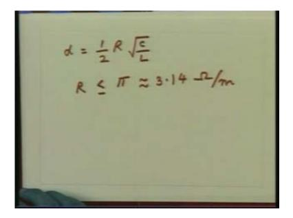
and if I substitute the value of  $\sqrt{\frac{C}{L}}$  and the value of  $\alpha$  which is  $\frac{\pi}{100}$  as you have taken one percent of the value of  $\beta$  then I get the value of R which is less than  $R=\pi$  approximately 3.14 ohms per meter.
