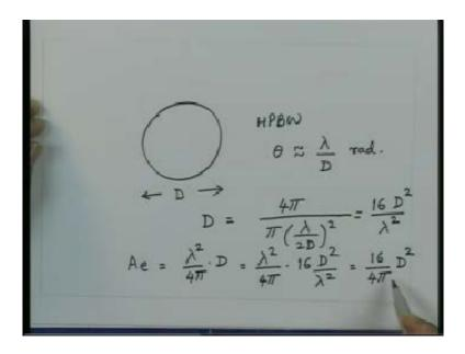
So if you see this quantity is close to about this square and so is the physical area if I calculate it is  $\pi$  upon 4 D square so this quantity is now very close or if I cancel this, this will become four so this will be equal to 4 D square upon  $\pi$ . So the physical area of this parabolic dish is very close to the effective aperture for this antenna.
