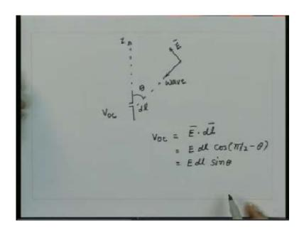
So if you recall precisely the same variation the antenna had while transmitting that is the radiation pattern of this antenna was  $\sin\theta$  for the Hertz Dipole so this quantity  $\sin\theta$  which tells me the variation of the open circuit voltage for this antenna as a function of the angle of the incoming uniform plane wave incident on this antenna that variation is  $\sin\theta$ . So we have a validation that is the radiation characteristic or what we call the radiation pattern
