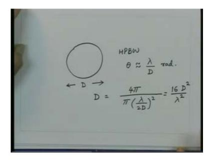
So what should be the effective aperture of this antenna A effective is  $\lambda$  square upon  $4\pi$  into D so that is equal to  $\lambda$  square upon  $4\pi$  into the directivity of the antenna which is
