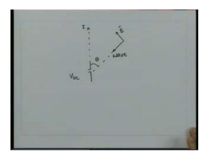
Now due to this electric field we have E dot dl so there is a voltage induced between this wire this is the Hertz Dipole and that is a dot product of dl which is the length of the dipole and the electric field. So as we can see from here the E dot dl the voltage  $v_{oc}$  will be equal to E dot dl where dl is the length of the antenna so here the length is dl, if this
