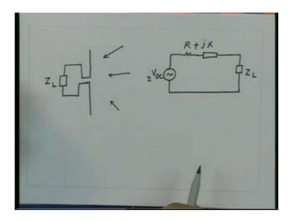
So if I see from circuit point of view, a receiving antenna is equivalent to an open circuit voltage that is the voltage which will measure between the open circuited terminals of the antenna the internal impedance of the antenna is the same impedance which you would measure between the terminals of the antenna when antenna is in transmitting mode and that is the load impedance to which finally the signal is delivered in the receiving mode.
