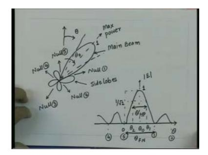
So we have the third characteristic parameter that is the beam width between first nulls we call that as BWFN.
