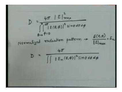
So if you know he normalized radiation pattern essentially you can calculate the directivity of a given antenna. Otherwise you can see from here essentially the directivity tells you the enhancement of the power density in a given direction with respect to an isotropic antenna. So this quantity by definition is always greater than one, for an isotropic antenna this quantity will be equal to one but any other antenna which is directional this quantity by definition has to be greater than one.
