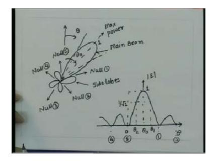
Then one can say if fifty percent variation of the power density is acceptable we can say effectively that is the angular sector over which your antenna beam is illuminating the region the power is going effectively over this sector. So we define this beam width  $\theta_1$  –  $\theta_2$  as the half power beam width of the antenna and that is the effective width over which the antenna is sending power along the main beam. So we have a second parameter called half power beam width.
