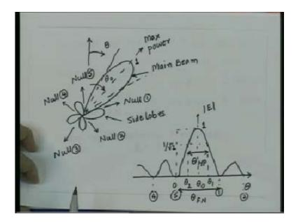
So we define this characteristic parameter called the side lobe level which is nothing but the larger side lobe amplitude divided by the main beam amplitude. (Refer Slide Time: 24:02 min)
