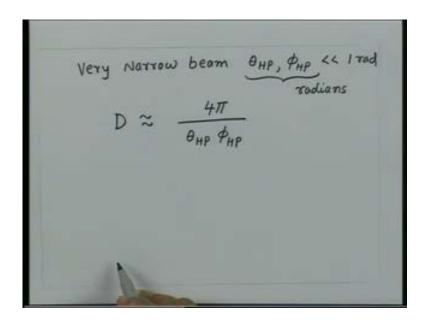
So if I could measure the half power beam width of an highly directional antenna then the calculation of approximate value of directivity is rather very straight forward. So that is why when ever we design an antenna if it is directional the first attempt is to measure half power beam width because once you measure the half power beam width then from there
