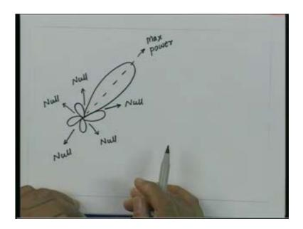
In this particular radiation pattern we have the direction in which the maximum power goes and there will be five directions in which no power goes the electric field is zero in this direction. Then if I go in this direction between these two nulls where the electric field is locally maximum so if I measure the magnetic field the magnitude of the electric
