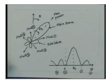
So essentially we can take the radiation pattern which is actually a polar plot in a plane as a Cartesian plot where the angle is plotted on the x axis and the amplitude of the electric field is plotted on the wires so this is I am plotting here |E|, both type of patterns are seen in literature some people prefer to draw the radiation pattern like this sometime when you want to do more calculations may be drawing the radiation pattern like this comes out to be more handy.
