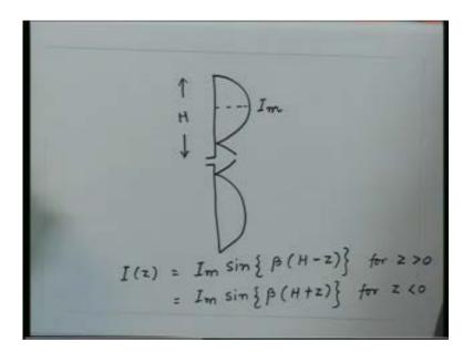
So this thing which you have written the current distribution now we can explicitly write this for the lower half of the dipole which is for z < 0 and for the upper half of the dipole which is for z > 0.
