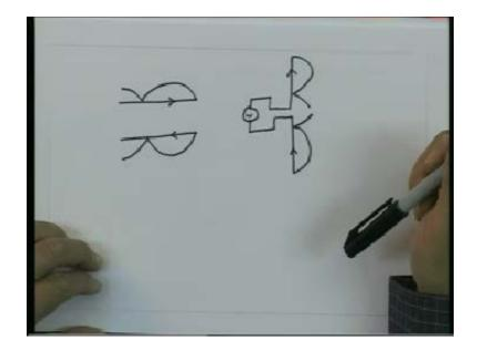
So we know the distribution that we can see from the flaring of photo transmission line also that means this is the standing wave when we have a sinusoidal distribution on this which is a standing wave pattern this pattern remains even when the antenna is completely flared up to become a dipole.
