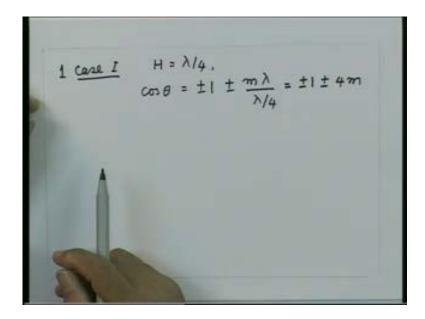
So if you are having a dipole of length  $\lambda/4$  then you get only the same nulls which are  $\theta = 0$  and  $\theta = \pi$ . So the dipole is of  $\lambda/2$  length so this length is  $\lambda/2$  and there are only two nulls one is in this direction other one is in this direction.
