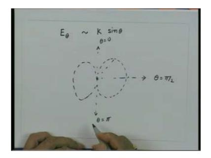
So if I visualize this in three dimensions then the structure essentially would look something like that. Here the antenna its size and all that are not given or not shown what is shown is the antenna is taken as a point and the field which is coming from that point are having a variation  $\sin\theta$  so I plot the amplitude of the electric field as a function of  $\theta$  and  $\phi$  I will create a surface which will look something like apple.
