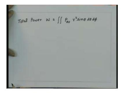
So what we have is we have Hertz Dipole here, we are considering a sphere around it of radius r so the incremental surface area on the surface of the sphere is r square  $\sin\theta \ d\theta \ d\phi$ .
