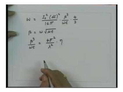
If I rearrange some terms into this and substitute, for that I will get the total power radiated by the Hertz Dipole that can be written in terms of the intrinsic impedance substituted here and if I take the radiation is taking place in the free space this quantity is  $120\pi$ . So this one you know for the free space is  $120\pi$  so I can substitute here for  $120\pi$ .
