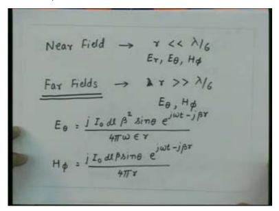
We can also see some interesting things from here and that is the electric and the transverse nature of the electromagnetic wave is there at every point in space and its direction will be changing when you go to different locations but at a given point how the electric field is varying as a function of time.
