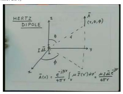
So the magnetic vector potential at a distance r from the origin essentially is given by this which we wrote explicitly as the z component which was essentially given by that.
