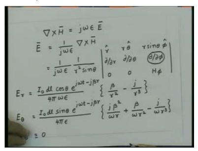
If I look at this term here which is beta upon omega r square, since beta is proportional to omega this term is independent of omega and this term is inversely proportional to omega. So this field induction field is independent of omega and this field electrostatic field whatever we are calling which is varying as 1 over r cube this is inversely proportional to omega 1 upon omega.
