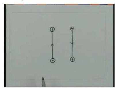
So essentially this current flow which we are talking about which is time varying is equivalent to having time varying charges which are accumulated at the two ends of this this current element which is saying that I am having an electric dipole whose charges are
