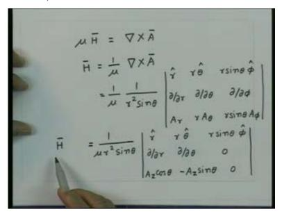
So the vector magnetic field essentially is given by the determinant which is this. Now it is immediately clear that since these two elements are 0 here the r component and the theta component are identically 0. The only component which you will get will be corresponding to the phi component which will be d by dr of this quantity minus d by d theta of this quantity (Refer Slide Time: 9:33).
