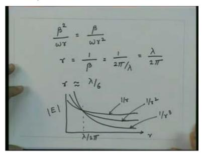
As we see as we go to lower and lower frequencies this is the term which will dominate. So if I go very close to the hertz dipole essentially the influence will be only the electrostatic field. If I am somewhere in between then I will get the induction field and if I go very far away from the dipole very far away means much much larger compared to lambda by 6 then practically the radiation fields will be present in the in the medium.
