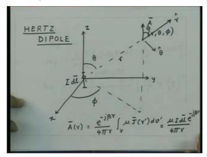
Once we get the magnetic field then we can go to the Maxwell's equation and now we want to find out the electric field not at a location of the source but somewhere in the space where there are no charges or no sources so essentially we can substitute the magnetic field in the source free Maxwell's equation and then find out what is the electric field.
