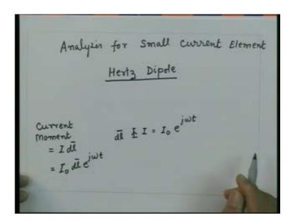
So, we carry out the analysis for small current element. This small current element many times as referred as the hertz dipole and the meaning of this will become clear in a short while from now. So, this thing is also called the hertz dipole. So, without worrying about how the current is again excited, in the current, in this small element, let us say I have a
