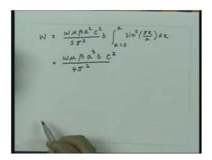
So I can combine these terms and get the total power inside the waveguide w that is omega mu beta a square c square upon 2 phi square, the integral with respect to y will be b. So multiplied by b integral x equal to 0 to a sin square phi x by a into dx and this integral will be only having a value of half. So you can get finally the expression which is omega mu beta a cube b, c square upon 4 phi square.
