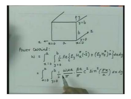
Again we use the same argument since at every location the field is going to vary as a function of times sinusoidally. We take the peak value of the magnetic field and just take the RMS value from there and then, you calculate what is the power loss by integrating over the length of the waveguide.
