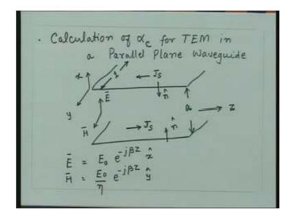
We have seen the calculation of these losses from the knowledge of resistance and the conductance in the transmission line. However, one may ask a question how do we know this resistance and conductance in the transmission line. So essentially starting from the fields we can calculate how the losses are going to take place in this conducting surfaces.
