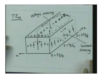
Now the field in x direction is having a sinusoidal variation. It is 0 here, it is maximum half wave and then is zero here again; and it is having a sinusoidal variation in the z direction with maximum at this location, which is Lambda g by 4. And then, if I go distance of Lambda g by 4 from here that means at z equal to Lambda g by 2, this quantity will go to 0. Then the fields will reverse and so on.
