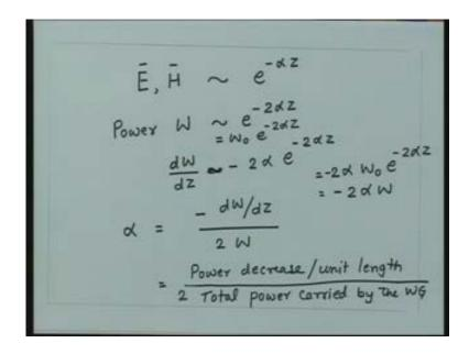
So the power which is proportional to mode e square or mode h square because power will be e cross h. So the power density or power which the waveguide carries or as the structure carries, let us say that is w that varies as e to the power minus 2 alpha z. I can differentiate this w with respect to z, so I get dw by dz that is equal to minus 2 alpha e to the power minus 2 alpha z. So w varies like this, so the dw by dz will vary like that instead of putting equal to let us say proportionality.
