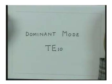
We also argued that most of the time, people want to operate in the dominant mode or in single mode on a waveguide to avoid the dispersion, that is broadening of that signal in time domain, as it travels on a guiding structure. So, this mode which is the dominant mode the T E 1 0 mode is the important mode for rectangular waveguide because most of the time the energy is going to propagate in this mode. So, whether you conduct the
