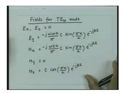
We have derived these fields and we have written these fields in these components. We have seen for a rectangular waveguide the E x and E z components are 0, the electric field has only y component which is given by this and the magnetic fields had two components which was, one was x component, other one was z component. So, there was no y
