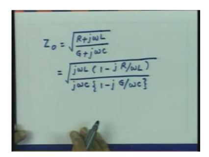
This quantity is  $\sqrt{\frac{L}{C}}$  that will be nothing but the characteristic impedance of the ideal Transmission Line I can expand this parameters again and this we can write as  $\sqrt{\frac{L}{C}}$  this square root again since  $\frac{R}{\omega L}$  is very small this can be approximated by  $1 - j\frac{R}{2\omega L}$  this will be  $1 - j\frac{G}{2\omega C}$ .
