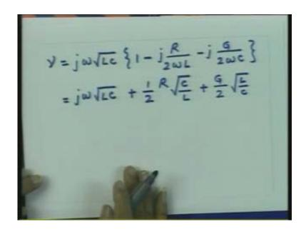
So this quantity here which is the imaginary part of the propagation constant that represents  $\beta$  and this quantity here represents the attenuation constant  $\alpha$ .
