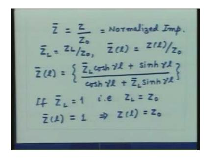
Now what we are saying is that if the load impedance is not equal to the characteristic impedance then the impedance measured at any point on the line will be the function of the length of the line or the input impedance of the line is the function of the length and the impedance which is connected to the other end of the line.
