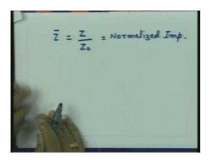
Then my  $\overline{Z}_L$  bar is equal to  $Z_L/Z_0$ , normalized impedance at any location 1 is equal to  $Z(1)/Z_0$  and so on.
