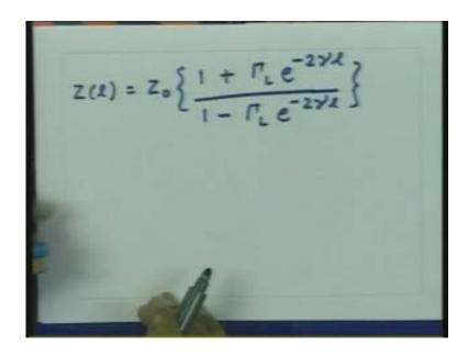
and  $\Gamma_L$  is nothing but the reflection coefficient at the load end so  $\Gamma_L$  as we have already derived is nothing but  $\frac{Z(1)-Z_0}{Z(1)+Z_0}$  where  $Z_L$  is the load impedance.
