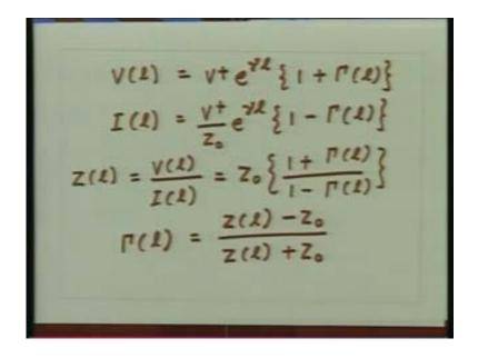
I can take  $V^+$   $e^{\gamma l}$  common so this quantity will become  $\frac{V^-e^{-\gamma l}}{V^+e^{\gamma l}}$  that is nothing but reflection coefficient at distance l. So I get  $V(l) = V^+$   $e^{\gamma l}$   $\{1 + \Gamma(l)\}$  and the current at that location will be  $\frac{V_0}{Z_0}$   $e^{\gamma l}$   $\{1 - \Gamma(l)\}$ .
