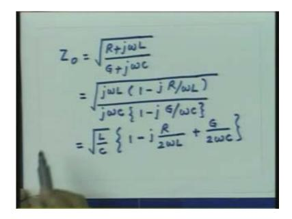
So the characteristic impedance this quantity is real by  $\sqrt{\frac{L}{C}}$  which is nothing but the characteristic impedance of the Loss-Less Transmission Line. But now for a real low loss line the characteristic impedance is no more real it has a component which is imaginary coming from this quantity there is some j here. So now we conclude two important things
