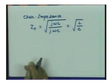
So the characteristic impedance of the lossless line is square root of the ratio of the inductance and the capacitance per unit length. But now the important thing to note is that for a lossless line this quantity is a real quantity  $Z_0$  is real and that is very interesting.
