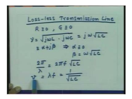
And from our basic physics we know frequency times the wavelength that is nothing but the velocity of the wave the voltage wave on Transmission Line. So the velocity of the wave is related to the inductance and capacitance per unit length on the Transmission Line so once the inductances and capacitances are given the velocity of the wave on the Transmission Line is reached.
