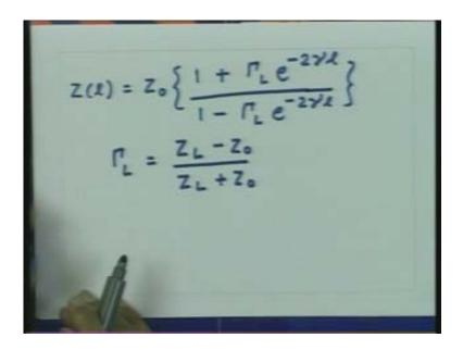
I can substitute for  $\Gamma_L$  into this equation and I can get the impedance at any point on the line in relation to the load impedance so I get a relation Z(l) called the impedance
