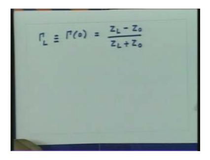
so what we find here is the reflection coefficient at the load end which is the measure of how much energy is reflected from the load end related to the terminating impedance of the line which is  $Z_L$ , also it depends upon the characteristic impedance of the line.
