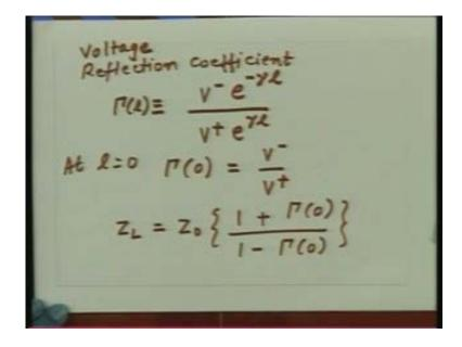
Both these quantities are complex in nature and that is the reason the reflection coefficient at any point on the Transmission Line is complex. Then at l=0 which means at load end the reflection coefficient which is  $\Gamma(0)=\frac{V^-}{V^+}$  so the ratio of the reflected and the incident voltage at the load end is denoted by this quantity  $\Gamma(0)$  at l=0. By substituting this we got the relationship between the load impedance and the reflection coefficient at the load end.
