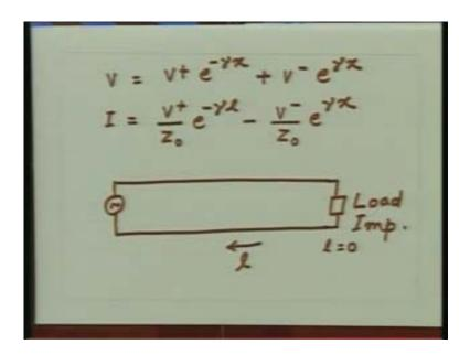
Then satisfying the boundary condition at the load end we got the relationship between the impedance at the load end which is related to the parameter which again was a ratio
