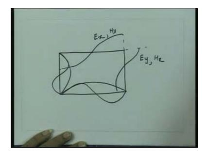
So in this case, the longitudinal component which we have is  $H_z$  which is like that and what is observed from this is that this component which is going to be tangential to this wall, this wall, this wall and this wall should be maximum on the walls and it should have a variation which is sinusoidal variation in the transverse direction.
