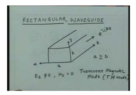
But the field has to be 0 here, this is  $E_z$  component; so it has to be 0 here, it has to be 0 here and there should not be any variation in the x direction if m is equal to 0. That is only possible provided the field is identically 0 everywhere; the same is true for these two boundaries that when n is equal to 0, the field should not have any variation in the y direction but it should be 0 here, it should be 0 here and that again can happen when the field is identically 0 everywhere.
