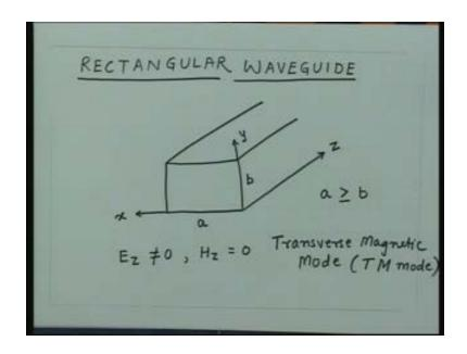
So, if I take the wave equation in Cartesian coordinate system, this  $E_z$  is a scalar quantity. So, we can write down the wave equation which is del square  $E_z$  plus omega square mu epsilon  $E_z$  that is equal to 0. This is the wave equation.
