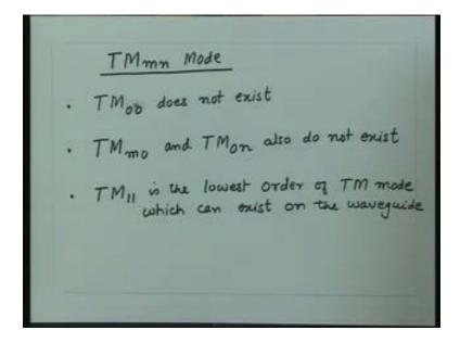
So, the first conclusion which we have is  $TM_{00}$  does not exist. So, we also conclude that  $TM_{m0}$  and  $TM_{0n}$  also do not exist. So, the lowest mode which can exist, the lowest index that is when both these indices are non-zero, that means  $TM_{11}$  is the lowest order of TM mode which can exist on the waveguide.
