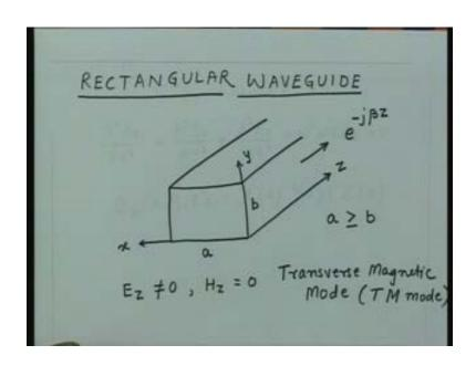
So this component, easier component is a tangential component to all the 4 walls of this and that is why we have 4 boundary conditions; one on this wall which is x equal to 0, one on this wall which is x equal to a, one on this wall which is y equal to 0 and one on this wall which is y equal to b.
