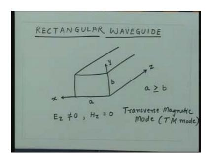
So, we have a wave guiding structure for which we have a hollow pipe whose cross section is rectangular and the energy is going to flow along the length of this metal pipe. We are again considering that this pipe is made of ideal conductor terminal conductivity of this pipe is infinite and the medium which is filling this wave guide is ideal dielectric. That means the conductivity of the medium which is filling this pipe is 0.
