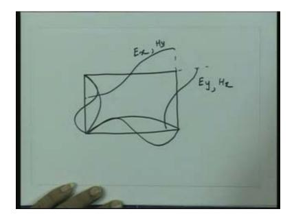
This will be the component which is  $E_x$ ; so that is maximum here, 0 here, maximum here and  $H_y$  component if I look at, it will be again a cos variation along y direction. So, it will be in this direction; if I look at, the field variation would be like that for the  $E_y$  component.
