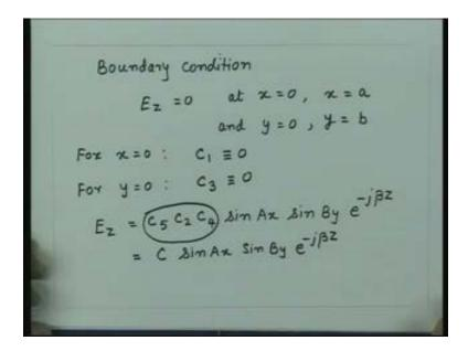
So, the  $E_z$  was 0 x direction at x equal to 0, at both the walls, the  $E_z$  was 0,  $E_z$  in y direction also having half cycle variations.
