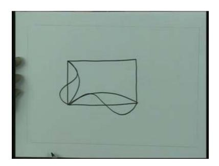
If I look at the cross section like that, the wave guide; the  $E_z$  is 0 here, 0 here, 0 here. So, it had half cycle variation like that or it could have a variation which will be like that, the same is true for half cycle variation in this direction or it could be like that. So, the  $E_z$  is 0 at this point and the maximum here if m is equal to 1, maximum here along this if n is equal to 1 and so on.
