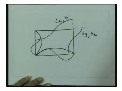
Now, this you can verify when x is equal to 0, the field is maximum; when x is equal to a, again the field is maximum; y is equal to 0 and again y equal to b, again the fields are maximum.
