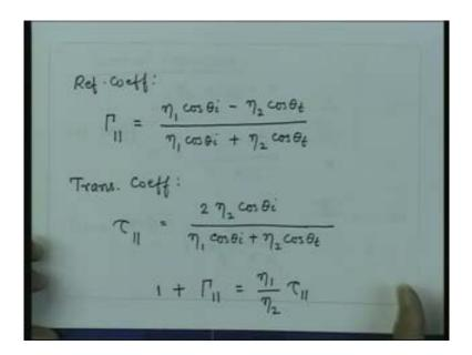
But if I go here which is for the parallel polarization and if I substitute theta i equal to 0 and theta t equal to 0. I get a reflection coefficient gamma parallel which is eta 1 minus eta 2 upon eta 1 plus eta 2. One would than wonder if I said by when theta goes to 0 2 cases should become identical why the reflection coefficients are opposite of each other.
