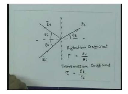
We are having same situation here that when the wave travels in this medium it suddenly sees a change in the intrinsic impedance and because of that impedance discontinuity the part of the energy gets reflected and we want to know what is the reflection coefficient which is ratio of  $E_r$  and  $E_i$ .
