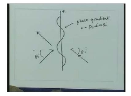
Now if I want to maintain the continuity of the electric and the magnetic fields both but once the electric and magnetic fields are induced into second medium they see infinite medium ahead of it that means again they constitute a wave phenomenon and since the medium seen ahead of them is infinite medium they again see a transverse electromagnetic behavior for the wave.
