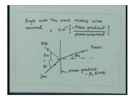
So what I can do is if I see in Medium 1 I can substitute this phase gradient value and sine inverse of that quantity or sine of this angle will be equal to the minus of phase gradient divided by the phase constant.
