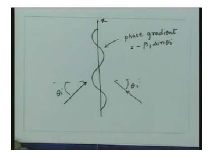
So whether the wave is coming this way on the interface or the wave is coming this way from the interface both are going to create identically same phase gradient. So the wave which was traveling through interface like this will correspond to this phase gradient, if the wave was passing through the interface like this it will create the wave gradient which is like this.
