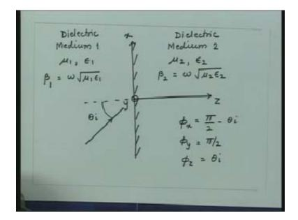
So I know in both media the phase constant for a plane wave and we know the angle which the wave vector makes with the three coordinate axes. So let us say I have some field represented by this wave which is having a vector and the phase function will be given as we saw last time as follows.
