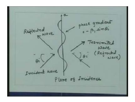
So now we have something important conclusions, when the uniform plane wave is incident on a dielectric interface at an angle we induce two waves in which one is called Reflected wave which is going away from the interface Medium 1, we induce another wave which is Transmitted wave which is going away from the interface Medium 2.
