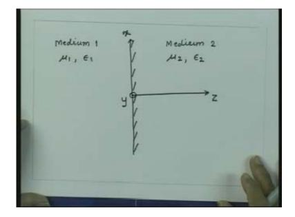
Now let us say we have a wave which is incident on this dielectric interface at some arbitrary angle with respect to the coordinate axis. So I have a wave which is incident at some arbitrary angle like that, this is the direction of the wave so essentially this is the wave vector for the wave which is incident on the dielectric.
