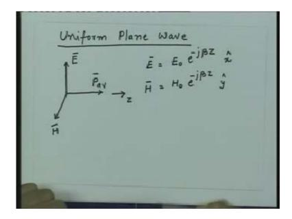
So the average Poynting vector associated with this  $\overline{P}_{av}$  is equal to the half real part of  $E \times H^*$ , now the cross product of x and y will give my direction z so this average Poynting vector is in z direction so this is half of real part of this conjugate so essentially that will become  $E_0H_0$  so this will give me  $E_0H_0$  in the direction  $\hat{z}$ .
