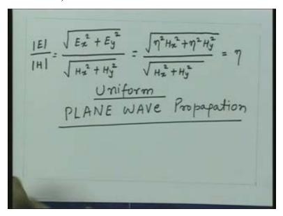
Magnitude of the magnetic field will be  $H_x$  square plus  $H_y$  square. So, if I say I take a ratio of the magnitude of the electric and magnetic field at any point then I get this. I can substitute for  $E_x$  and  $H_y$ , I can get here this is square root of eta square  $H_x$  square plus eta square  $H_y$  square divided by square root of  $H_x$  square plus  $H_y$  square that is equal to eta.
