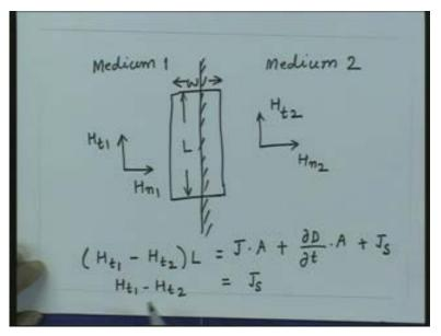
If there is no surface current density then the different between the tangential components of magnetic field will be equal to zero. Or in other words, the tangential component of magnetic field also will be continuous across the boundary. So, using these four Maxwell's equations in the integral form applied to media interface we get the so-called boundary conditions.
