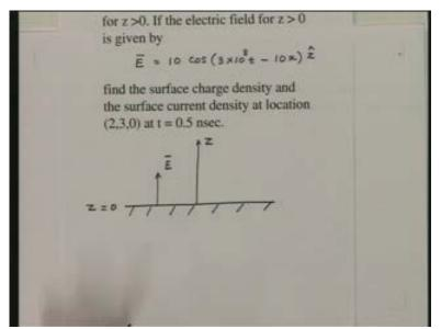
Now the surface charge density essentially is related to the normal component of the electric field. Now in this case the electric field which is given here is already normal to this conducting surface so the surface charge density in this case rho s that will be equal to rho 0 epsilon 0 epsilon r into the normal component of the electric field E n.
