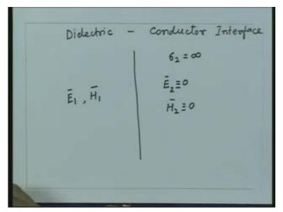
Then I can go back and apply the boundary conditions which I have got here which are in general. So since this quantity is electric field is 0 in this medium and epsilon times or the permittivity times the electric field is the displacement vector so D n2 is identically 0 inside the conductor.
