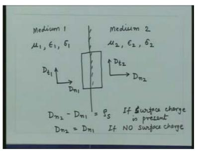
So this is one boundary condition which we have from the Gauss' law that the normal component of the displacement vector is continuous across a boundary if there is no surface charge and in the presence of surface charge the difference of the normal component of the displacement vector is equal to this surface charge density. This is this is boundary condition 1. So we have a boundary condition on the normal component of the charge density.
