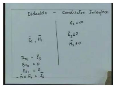
So depending upon the situation whether we have the dielectric dielectric interface or we have dielectric conductor interface we can appropriately apply these boundary conditions. This now gives us the framework for analyzing any electromagnetic problems in three dimensional space.
