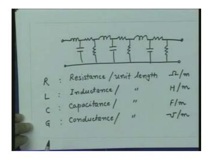
Now I have defined these quantities which we call as the Primary constants of the line which are the values of the Resistance, Inductance, Capacitance and Conductance per unit length of line. So these parameters are called the Primary constants of the line. So for any transmission line we can define these primary constants.
