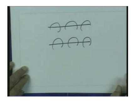
These magnetic fields linkage with the current that gives you the inductance of this wire and the separation between these two conductors by dielectric essentially gives you a capacitance between the two conductors. So we have an inductance along the conductance and we have the capacitances between the conductors. And this inductance or capacitance is not located at any point but they are distributed all along the length of this structure.
