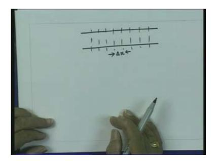
Then this small element can be represented by a combination of Inductance, Resistance, Capacitance and Conductance with appropriate values and since I know these values per unit length I can multiply that by  $\Delta x$ . So I know this value for this small element so this small section of the Transmission Line is equivalent to a Inductance, a Resistance, a Capacitance and a Conductance and the value of this will be the value of the line per unit length multiplied by the length.
