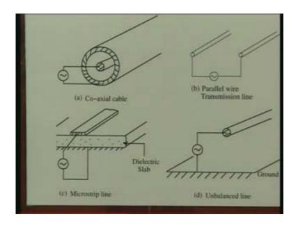
We can have a structure where the two conducting wires or rods can run parallel to each other. We can apply a voltage between these two rods and the energy will flow along the rods.
