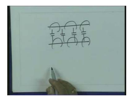
These parameters are called the distributed parameters of the line and the analysis which we are going to carry out for the Transmission Line is called a distributed circuit analysis. So these elements are called the Distributed Elements.
