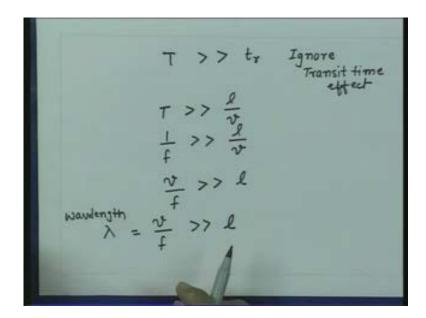
So if the wavelength of a signal or the voltage which is I am applying across the line is much larger compared to the physical size of the line then the Transit time effects can be ignored. However whenever the wavelength becomes comparable to the physical size of the element then the Transit time effects cannot be ignored I have to take the Transit time effect into consideration.
