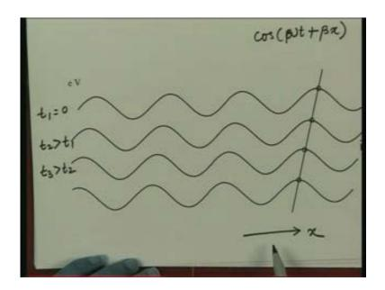
Now in this case when your function is the second term of the solution where the function is  $\cos(\omega t + \beta x)$  the point will appear moving leftward or in the negative x direction but in both the cases the phenomena appears to be moving on the Transmission Line. So what we see in general is that as soon as we introduce a Transit time effects on the Transmission Line the voltages and so will happen to the current will exist in the form of traveling waves on the Transmission Line.
