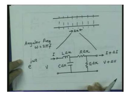
So, at any location if I find out the voltage and current varying sinusoidally as a function of time with an angular frequency  $\omega$ , so if you have to get the instantaneous value of the voltage and current at any location and at any time essentially this value of voltage and current has to be multiplied by  $e^{j\omega t}$  so we get the instantaneous value of the voltage at that location.
