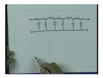
Now if I measure this quantity the inductance per unit length of the line which is the value of the distributed element per unit length same is true for Resistance, Capacitance, and Conductance and so on.
