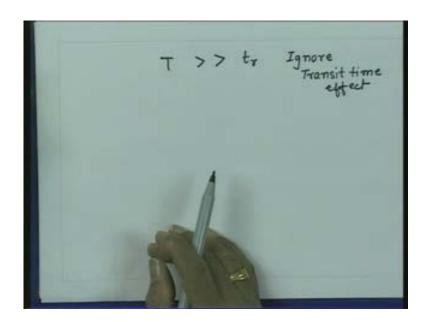
However when T becomes comparable to the Transit time that time we have to incorporate the Transit time effect into the circuit analysis. I can substitute for the T and the Transit time from here so  $T = \frac{1}{f}$ , the Transit time is length of the line divide by the velocity so the condition is,
