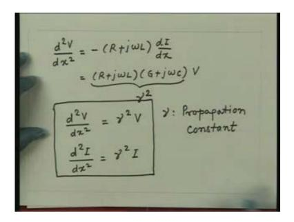
so I get  $(R + j\omega L)(G + j\omega C)V$  where the two negative sign cancels each other and say you have positive sign here. Now this quantity whatever it is, is some kind of a characteristic quantity for a Transmission Line because it depends upon Primary constants of Transmission Line R, L, G and C and it is also depends upon the frequency of operation.
