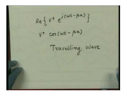
because  $V^+$  is the real quantity that is what we assume,  $\cos(\omega t - \beta x)$ . So if I take some value of t and vary x I will get a function which will be sinusoidal function, if I change the value of t to some positive value I will get another function which will be shifted in x. so if I look at this function, this function essentially in space will look like
