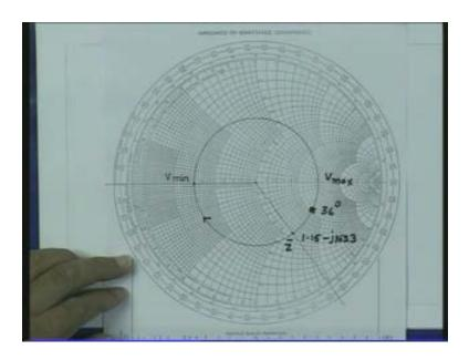
So essentially from the maximum location if I move away from the generator that means in the anticlockwise direction by an angle of 324 degrees on this constant VSWR circle whatever point I reach to that point corresponds to the load impedance. If I make a moment like this by 324 degrees I reach to this point. Now a if I read of the value of the normalize resistance and reactance corresponding to this point I get a value "1.15" minus j "1.23".
