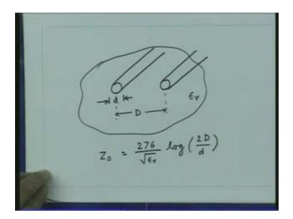
So Z 0 for this is be 276 ohms, so as we can see for this structure realizing low impedance is more difficult. I cannot realize to impedance a lower than "82.8" ohms. However, I can
