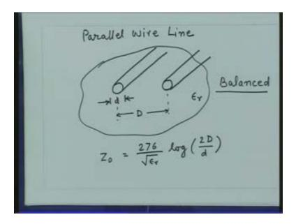
So this structure which is the parallel wire line this structure is a balanced structure whereas if I take a line which is a coaxial line or the micro strip line then this structure is an unbalanced structure. So in practice you see both kind of lines, the balanced lines and unbalanced lines and whenever we make a connection between the balanced and unbalanced lines, 2 things are to be seen one is of course the impedance has to be match, so that there is no reflection from the junction.
