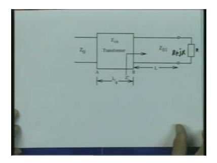
So it is possible to match a complex impedance R plus jx, so this impedance is R plus jx from here the principle is exactly same that if I get a impedance here which is real then, I can transform using quarter wavelength transformer, the impedance is to equal to Z naught.
