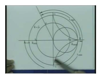
So normalization of this R plus jx is to be carried out with respect to this characteristic impedance. Once, I get this then as we move towards the generator, I move on the constant VSWR circle, if I reach to this point which is the right most point T on the constant VSWR circle then, the impedance here will be real and its value will be the VSWR. So the
