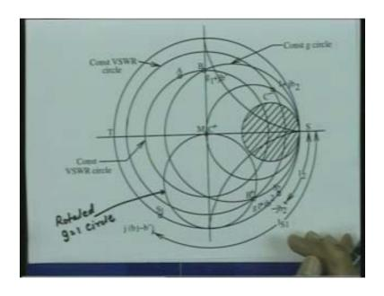
So the original admittance was g plus jb after transformation by a distance of 1 1, the admittance seen is g 1 plus jb prime which, when is combined with acceptance minus jb 1 you get a admittance here which is g 1 plus jb 1, which is when transform appears like a
