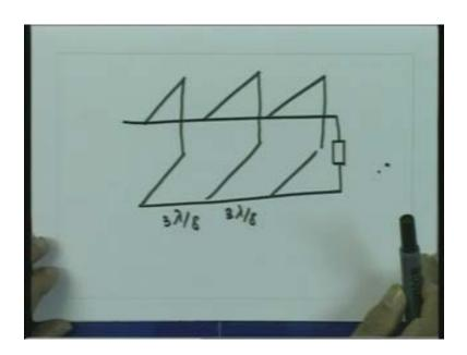
However, this thing has been taken away by introducing the concept simple which is the 3 step matching and that is, if I take this load, what we can do instead of using 2 stubs that we use 3 stubs, the distance between the all of them is 3 lambda by 8, this is 3 lambda by 8 and this is some value 1 1, what I can do is if because of these 2 stubs, the matching is again double stub but if the matching is done with these 2 stubs, I can make this open circuit by
