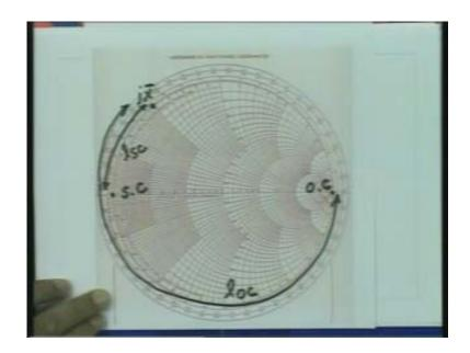
So depending upon the choice of the circuit we can either have the section of line which is open circuited or short circuited and we can realize that for any arbitrary inductance or capacitance on the Transmission Line.
