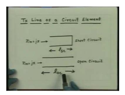
I know the value of the reactances at this location I know the value of impedance at this location which is either short circuit or open circuit and I want to find out what should be
