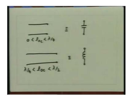
Now any section of a transmission line of size from zero to  $\lambda/2$  can realize any arbitrary value of capacitance and inductance at a given frequency. Let me again mention that we are not realizing an inductance and capacitance we are realizing the inductive or capacitive reactance and equivalently we can say that the reactance is having that capacitance or that inductance.
