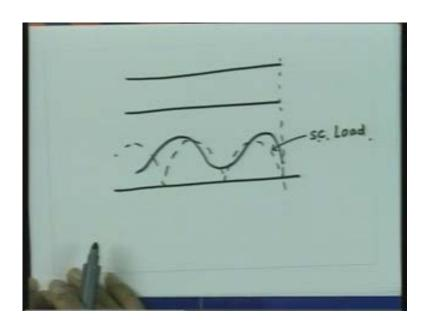
So I have two patterns here. This is for the load, this for short circuit and now this is the location at which the load is either connected or the short circuit impedance is connected. As we know that the location which is at this location has been repeated at every  $\lambda/2$  distance so whether I do the measurement at this point or I do the measurement at this point or this point they are identical because the impedance characteristic repeats every  $\lambda/2$  distance.
