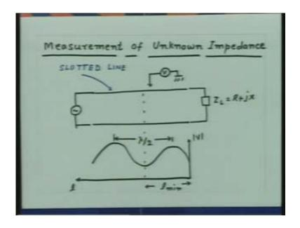
If you recall I had mentioned that when you go to high frequencies the measurement of phase is a very tedious task you can measure the amplitude of a signal rather reliably but the measurement of phase is rather unreliable. We have to measure the complex voltage and complex currents for measurement of complex impedances and since the measurement of phase is not that simple the measurement of complex impedance becomes very difficult at high frequencies.
