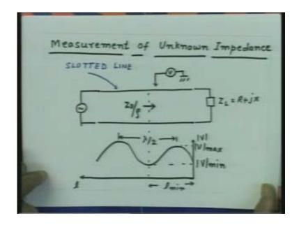
So from here now I calculate the quantity  $R_{min}$  which is the characteristic impedance divide by the VSWR  $\rho$ . Once I know the impedance at this location then the calculation of unknown impedance is simply an impedance transformation problem. As we had said if we know the impedance at any point on Transmission Line we can find the impedance at any other point on Transmission Line by using the impedance transformation relation.
