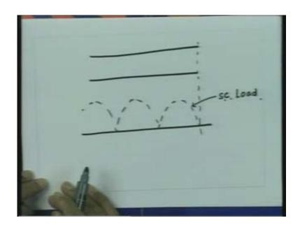
Now I replace this load by the actual load on the Transmission Line. Two things will happen the voltage standing wave pattern in general will be shifted with respect to the short circuited standing wave pattern and also the VSWR is not infinity so  $V_{min}$  voltage will not be zero. So in general we might get a voltage standing wave pattern which will look something like this. So now I may not have a maxima and minima of the short circuited pattern and this pattern at the same location.
