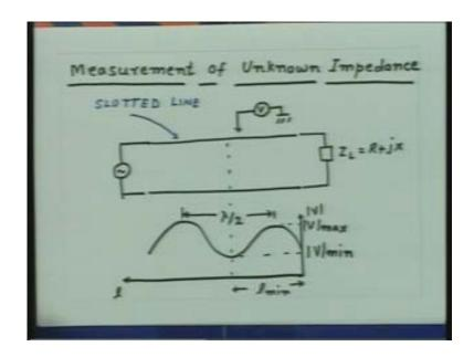
So now I have measured the propagation constant or the phase constant  $\beta$  on Transmission Line, measured the maximum and minimum voltage on Transmission Line and also the location of the voltage minimum on Transmission Line.
