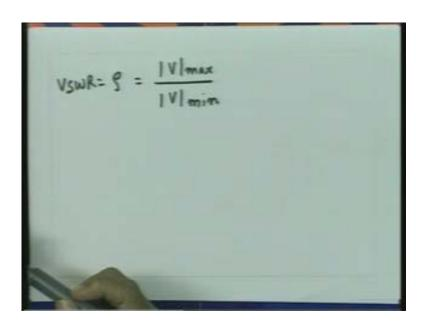
Once you get the VSWR  $\rho$  we now know the maximum and minimum impedance which one can see on Transmission Line. So at a location where the voltage is minimum that is this location here now the impedance will be the minimum impedance and that will be  $R_{min}$  and as we have seen earlier  $R_{min} = Z_0$  divide by the VSWR so I know the impedance at this location here that is  $Z_0$  divide by the VSWR.
