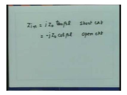
Getting this is very straight forward in the impedance transformation relationship if I put load impedance zero for the short circuit case I get the  $Z_{in}$  which is the transform impedance over a length I towards the generator which will be the input impedance, if I take the open circuited line then I put load impedance equal to infinity then over a distance I towards the generator I get the input impedance which will be given by that.
