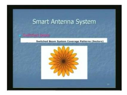
And one can transmit the signal or can receive the signal from that zone depending upon which area the observer is. So controlling the radiation characteristics is one of the important aspects of Antennas.
