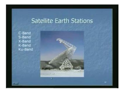
There are certain frequency bands assigned for Satellite communication called C-Band, S-Band, X-Band, K-Band and Ku-Band.
