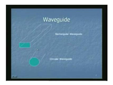
And in this process essentially we end up into a hollow pipe of metal inside where the electromagnetic waves can propagate. This structure is called a Waveguide.
