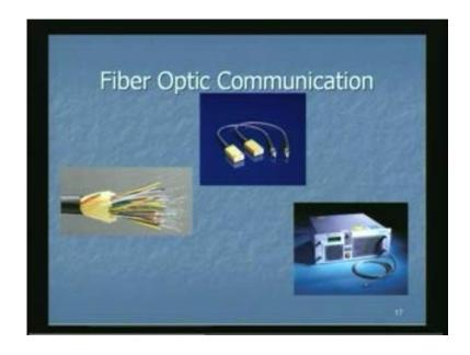
Here you can see a set of optical fibers having a very thin structure which is made of glass through the light is propagated. And we require a good theoretical understanding of propagation of light inside this because the signal gets distorted as the light propagates inside the Optical Fiber. Unless we understand fully how the signal get distorted one will not be able to tell how efficiently or properly the data can be transferred on this medium which is Optical Fiber.
