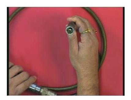
So electromagnetic energy propagates inside this and as I mentioned earlier these kinds of structures Transmission Lines are used at frequencies up to few Giga hertz.
