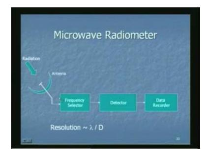
They are frequency converted, detected and processed. And again we would like to know precisely from which direction a radiation is coming or in other words by a Radio Telescope one would like to get an image of a sky with as larger resolution as possible. So again this resolution limit  $\frac{\lambda}{d}$  comes into picture and one requires very large telescopes to get a very fine resolution of the image of the sky.
