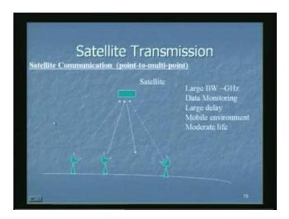
The satellite receives this signal converts its frequency and then sends it down towards the earth and this signal which is coming towards the earth can be received by the receiving stations on the earth. So one can establish a communication between one point on earth to any other point on earth. This whole propagation of electromagnetic radiation and proper placing of radiation in a direction towards the earth is controlled by the electromagnetic wave phenomena.
