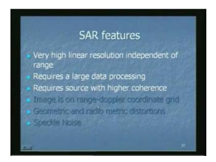
Firstly, you get a very high linear resolution from this Radar which is independent of the range though it requires very large atom processing. So electromagnetic waves find very active application in investigation of Synthetic Aperture Radars.
