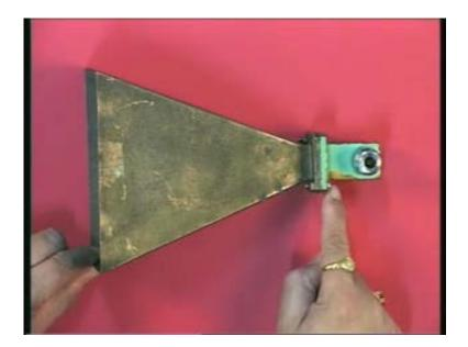
So electromagnetic energy is connected at this point, these are sides this structure which is the wave guiding structure and then my flaring this wave guide in this shape essentially the radiation goes into the space. So this device is an antenna which is normally used at microwave frequencies.
