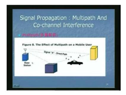
So again you require good design of the antenna systems which again require a good knowledge of electromagnetic waves so that the multi path interference in a mobile communication can be reduced.
