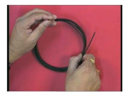
and the light can now go through this structure can emerge very efficiently from the other end of the fiber. So the electromagnetic wave in the form of light can be sent over very long distances by using optical fibers.
