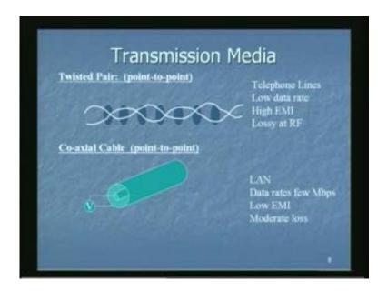
Now we will see this kind of medium is normally used for Telephone Lines and we want to investigate how the electrical signals will propagate on this structure. This media the twisted pair can handle low data rates, has a high Electromagnetic Interference and is very lossy as the frequency increases. So normally this medium is very useful for low frequencies but as the frequency increases the loss increases and that is why this medium became not very attractive.
