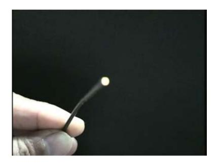
This is another optical fiber which we have here, this is very thin typically of the order of about 125 micron so the thickness is little thicker than hair.
