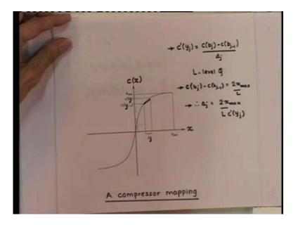
Now, in the earlier class we had seen that a compressor mapping in general has the following characteristics and if the interval is very small for very high rates. Then the derivative at reconstruction level y j can be approximated by this expression and then c of b j minus c b j minus 1 itself is equal to 2 x max upon L in which case, the delta j is equal to this expression out here. So, this we had seen in the earlier class we will use this result and substitute in this expression out here.
