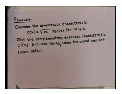
Now, let us take one more example, suppose we had the compression characteristics given by this expression, and it is desired to find the complementary expander characteristics that is c inverse x. We are required to evaluate signal to quantization noise ratio when the signal has P D F shown below it is of this form. So, let us try to find the solution to this again.
