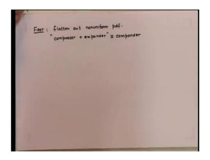
So, first let us try to flatten out the non uniform P D F using the following compressor and expander, which together is known as compander.
