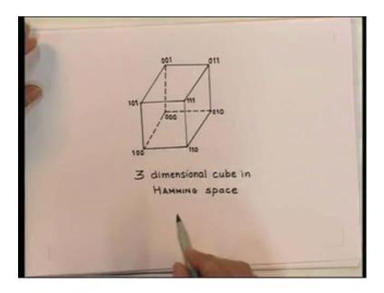
This is a 3 dimensional cube in hamming sphere. This is a three dimensional cube in hamming space. It is convenient to map binary sequences as shown in this figure and to talk in terms of what is called the hamming distance.
