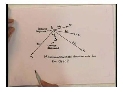
Beta j is the received sequence and alphas are the transmitted sequence. So, in this figure, beta j is closest to the code word alpha star where the distance is indicated by small d which is the smallest distance compared to all d i j's.
