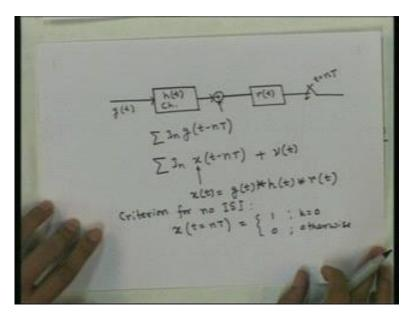
Once it goes through the channel with the impulse response ht channel filter and of course, there is noise. And then, at the receiver we implement some matched filter receiver. Now, this is the let us say this is baseband pulse and there is the received filter at the output of which we sample every t seconds. So, this is sampled at multiples of T
