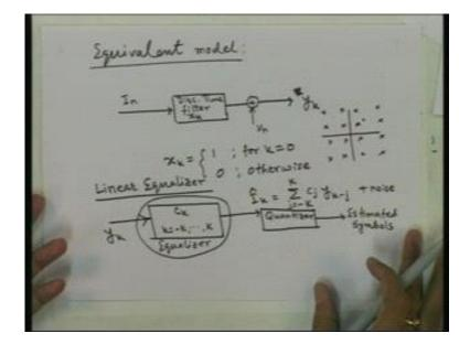
So, the equivalent model of the system becomes In and there is a discrete time filter with impulse response xk and there is some noise discrete noise. And here we have yk and our job at receiver will be to cancel the effect of this filtering and recover what was transmitted.
