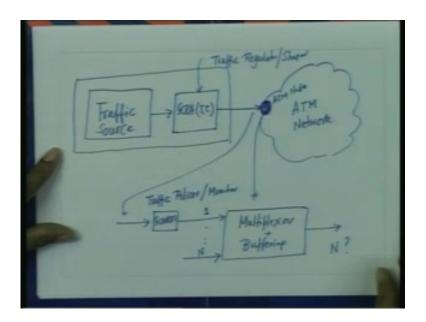
So in practice, basically, what we are doing is we are putting. So, here is a traffic source here is a traffic source. This traffic source passes through a GCRA (T, tau) and here is ATM traffic. So, this now of course to some kind of an ATM network.
