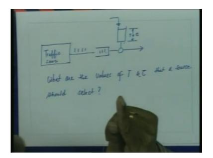
So now, what is the situation here? The situation here is that here is a traffic source which is transmitting these cells and they make pass, this traffic GCRA (T, tau) is essentially is a leaky bucket and as we had considered this leaky bucket has a depth of T plus tau; the fluid is accumulating at a unit rate and then the sources is transmitting and it has a bucket depth of T plus tau.
