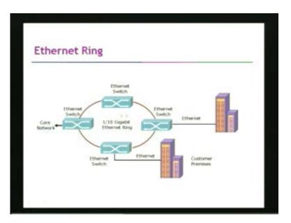
So, this is like an ethernet ring which is shown here. So, these are all Ethernet switches. These Ethernet switches are connected together in a ring form and these rings could be either 1 gigabit Ethernet ring or it could be a 10 gigabit Ethernet rings and from this switch, you can give ethernet based connections to directly to a customer premises and also from here.
