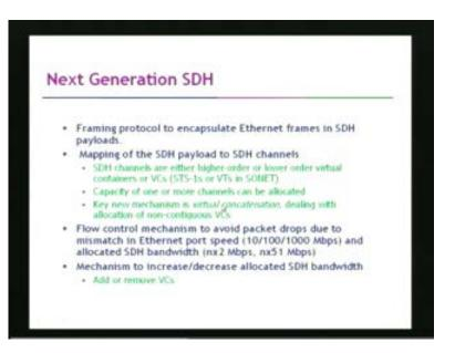
Now, next generation SONET or SDH is like a one step forward from the traditional SDH based networks. Now, next generation SONET SDH is basically is really a framing protocol which allows to encapsulate ethernet frames in the SDH payloads. So really, next generation SDH provides you a mechanism of encapsulating ethernet frames in the SDH payload and then tells you mapping of the SDH payloads to SDH channels.
