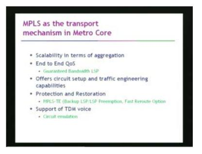
Now, MPLS as the transport mechanism in metro core has lot of advantages. It can provide scalability in terms of aggregation. MPLS can of course give you end to end quality of service guarantees in terms of guaranteed bandwidth label switch path, it can offers a circuit setup and traffic engineering capabilities.
