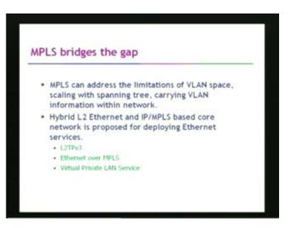
The solution it turns out is that the MPLS, the multi protocol label switching actually bridges the gap. We have already studied MPLS in our previous lectures and now we will see how MPLS can really be a useful device, can be a useful technology for addressing this challenge that we can have a ethernet based broadband access deployment using MPLS as the transport technology in the core of the networks.
