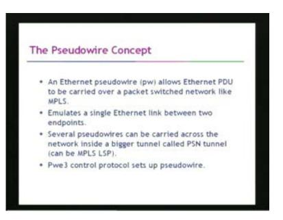
There is this pseudo wire concept; an Ethernet pseudo wire will allow an Ethernet PDU to be carried over a packet switch networks like MPLS and it basically emulates a single Ethernet links between 2 points and several pseudo wires can be carried across the network inside a bigger tunnel which can be called as a MPLS label switch path.
