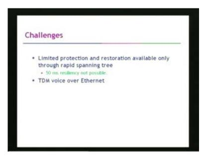
Then there is a limited protection and the restorations capability is 50 milliseconds, resiliency is not possible and finally we have the Ethernet based broadband networks typically cannot carry the TDM quality voice unlike in the SDH network, in the SONET SDH networks where it was possible to carry the TDM quality voice and as well as the packet data.
