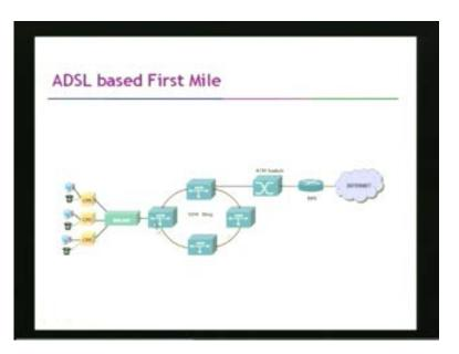
So, an ADSL networks would look something like this that in the first mile, you have a DSL access multiplexers which is called as a DSLAM. At the residential customers, you can have an ADSL CPE which is a customer premise equipments. These CPEs are connected to the DSLAMs and the DSLAMs can have an E 1, E 3 as an output and can get connected to an ADM in an SDH rings.
