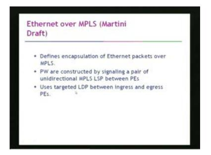
So, Martini draft actually defines the encapsulation of Ethernet packets over MPLS. Then pseudo wires are constructed by signaling a pair of unidirectional MPLS/LSPs between provider edges and then it uses target LDP between ingress and egress provider edge.
