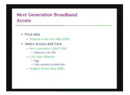
So, instead of using the traditional ADSL based or TDM centric architectures, we are proposing that ethernet be used in the first mile network which is called as EFM. As well as in the ethernet be used in the metro access and core. Now, in the metro access and core, there are 3 ways in which these Ethernet can be used.
