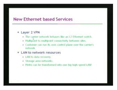
And, those new Ethernet based services are: one can have a layer 2 VPN, so the layer 2 VPN is like, so we can see that we have seen that a virtual typically, the corporate offices of a particular networks, they get connected through a service providers network at a layer 3 level and form a virtual private networks.
