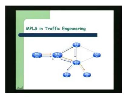
So here is an example of this that these are all you know labels which routers. So for example there may be um some traffic which may be going from this node to this node. So in a constraint based routing algorithms you know you may select some traffic to go on this link and that may be an optimal path for this but some traffic may get diverted onto this link.
