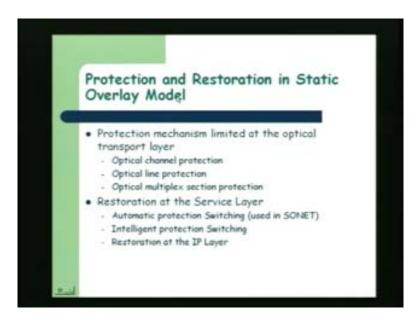
Now, if you consider the protection and restoration which is available in the static overlay model, then the protection mechanism is basically limited at the optical transport layer only if you see the static overlay model and there may be some restorations capabilities which may be available at service layer.
