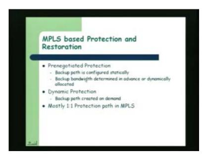
Now, how does this MPLS does these protections and the restoration will work? So, we are still talking in the context of overlay model only. So, we have at the edges those IP routers which are over layer over this optical cross connect or wavelength based routers. But now we are actually talking of restoration which will be available at the IP layer.
