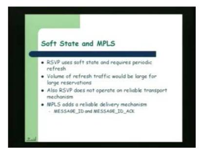
Now as we have seen actually, the RSVP is a soft reservation protocol in the sense that QoS state maintained by the RSVP are typically soft in the sense that they require periodic refresh mechanisms unlike in the atm world where the QoS signaling state could be a hard signaling state. In RSVP, the signaling state is typically soft and what is done is that it requires a periodic refresh mechanism. These QoS states need to be periodically refreshed.
