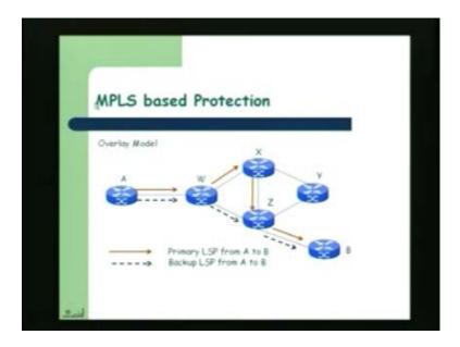
So, this is how MPLS based protection will operate. So, these are all, so here is the primer LSP from a to b which is shown in the red color here and here is a backup LSP which is shown from here. Now, in the normal course, the packets will be forwarded on this primary LSP that is this red line but let us say any of this links breaks down, then when this is discovered by this label edge router; then the packets will actually start forwarding on the back up LSP.
