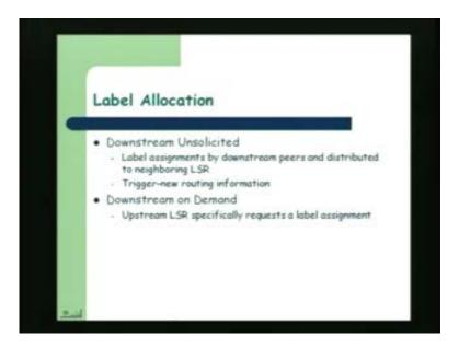
Now in downstream based label allocations, it could be of two types. Downstream Unsolicited: Now downstream in downstream unsolicited the label assignment is done by the downstream peers and then it is distributed to the neighboring LSRs. We had already discussed that we consider a node to be a downstream node with respect to another node if the packet flow is going to be in the opposite direction.
