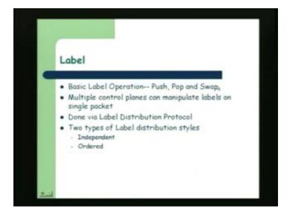
So now what are the basic operations which a label switch router will do? The label switch routers will do a basic operation on the label is push, pop and swap. So as you can see the swap
