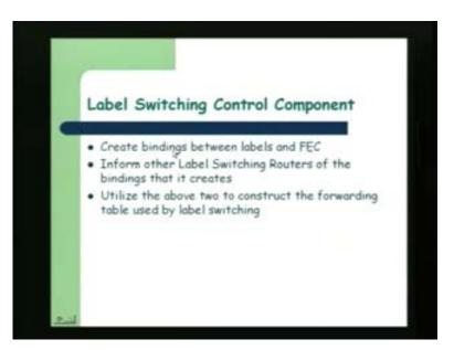
Now this control protocol will create the bindings between the labels and the FEC and then inform the other label switch routers of the bindings that it has created and then utilize the above two to construct the forwarding table used by the label switching.
