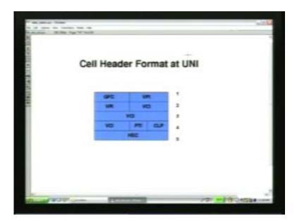
As we said that in ATM network, the cell, the packet consists of 5 bytes of headers. So, which you are seeing here, this is the 5 bytes of headers and we have 48 bytes of pay loads. So now, if you see here, VCI here which is 16 bit or 2 bytes of headers which is VCI. So, VCI stands for virtual circuit identifier VCI stands for virtual circuit identifier. Then we also have VPI. So, I will shortly tell you what is VPI. So, we will just see what are VPI and VCI.
