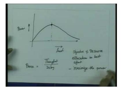
So, what we can say is that that we can plot offered load verses power and this power is nothing. The power of a flow is defined as the throughput upon delay. So, what happens is that if I keep on increasing the load, my power keeps on increasing and I reach a point and after that if I increase the load, my power actually decreases and eventually the power may become 0.
