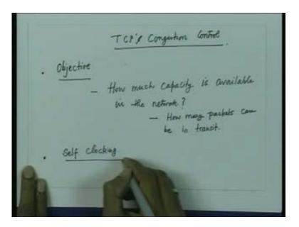
So, what we are saying is the TCP's congestion control mechanism. Now, the TCP's congestion control mechanism really works with an objective. It tries to determine how much capacity is available in the network. So, the TCP's congestion control mechanisms operates by saying how much capacity is available in the packet in the network and therefore how many packets can be injected into the network and the technique is essentially based upon the window based congestion control mechanisms.
