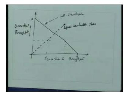
So, let me just show you that suppose if we try to plot the two connections throughput, so this is connection 1 or TCP connection 1 throughput verses connection 2 throughput. Now, if you see if you plot this line R; since R is the output link and if I plot this straight line, if you take any point on this line let us say if I take this point, then clearly here the connection one is nearing higher throughput, connection 2 but sum of the 2 throughputs is R.
