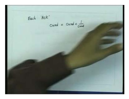
So, in a crude term we can say that every acknowledgment every acknowledgment, each Ack each Ack will adjust the window size, let us say CWnd is something like CWnd plus as measured in packets as measured in packets. So, if CWnd Acks have come, then the window size will by these by 1. But remember that the congestion window in TCP is measured in terms of bytes. So therefore, this is the correct equation where we are saying.
