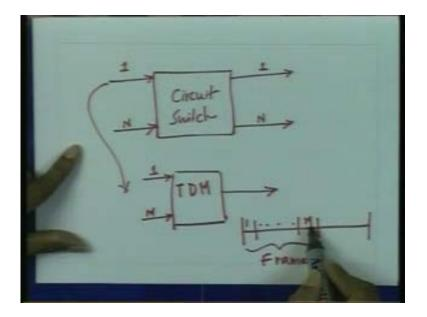
So, let me just explain what is meant by the circuit switching and the principal of time division multiplexing. Typically, in a time division multiplexing we will have multiplexers followed by a switch. So, let us say that this is a circuit switch which which could be an N cross N switch. So, where there are 1 to N input ports and 1 to N output ports.
