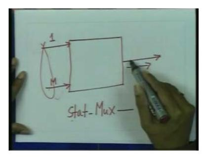
So, now what we are saying; here is the traffic source, each of this traffic sources and this each of this traffic source are characterized by this kind of probability density function. So, now we are saying that when these sources are multiplexed whether we can have some kind of admission control which can offer you quality of service guaranties.
