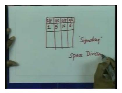
Now, the time signaling you know, this circuit switch will have some kind of a translation table which will look something like this that there is an input port, input slot, output port and output slot. So, you will say; what is the input port, what is the input slot, what is the output port, what is the output slot. So, that means typically in an input port of one input slot of let us say, 5 may have to be switched to output port of let us say, N and some output slot may be equal to 6.
