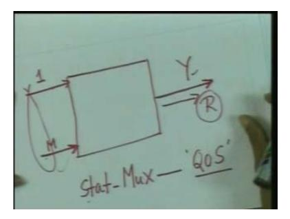
That means the R is the output link capacity of this.
