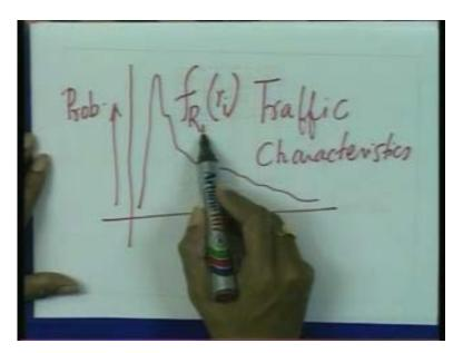
So, we can say that this is a density function, probability density function of a source whose bit rate in this case is  $R_i$ .
