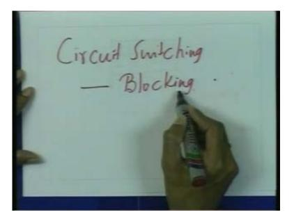
So, as we have seen, while circuit switching was characterized by blocking; by blocking I mean that if all the slots are occupied, then the users are blocked. If all the 32 slots in our time frame are occupied or or or all the M slots are occupied, then if N plus 1th user attempts to transmit, then he gets a busy tone or what we call he gets blocked.
